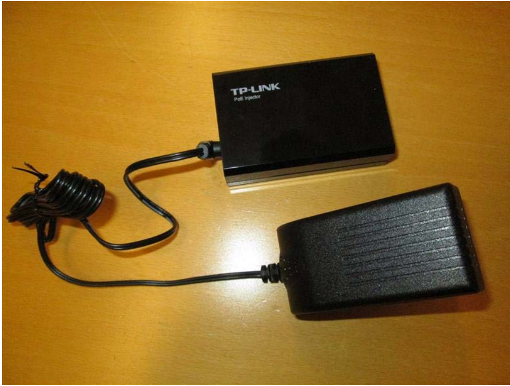
Photo 2.3.1 Auxiliary equipment. PoE injector with adaptor.
