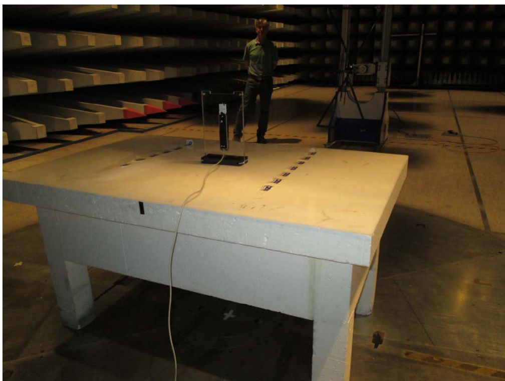
Photo 4.3.2 Test setup regarding measurement of radiated emission 30 – 1000 MHz
