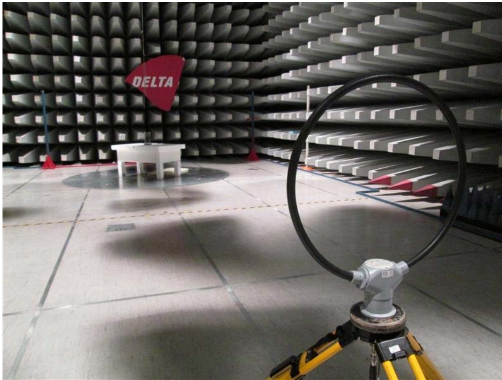
Photo 4.2.1 Test setup regarding measurement of radiated emission 9 kHz – 30 MHz. Antenna position X
