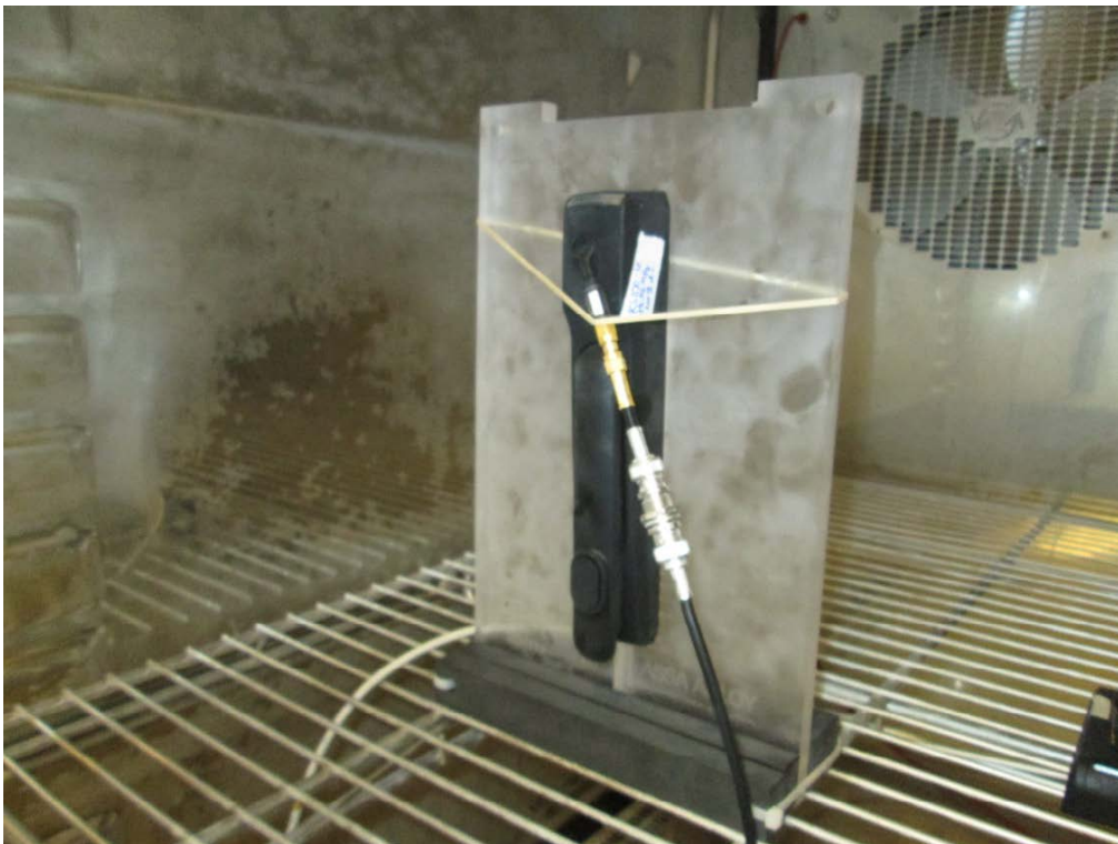
Photo 4.7.2 Test setup regarding measurement of carrier frequency stability. Test object in climate chamber.
