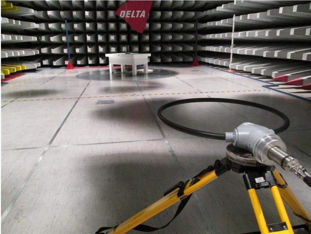
Photo 4.2.3 Test setup regarding measurement of radiated emission 9 kHz – 30 MHz Antenna position Z
