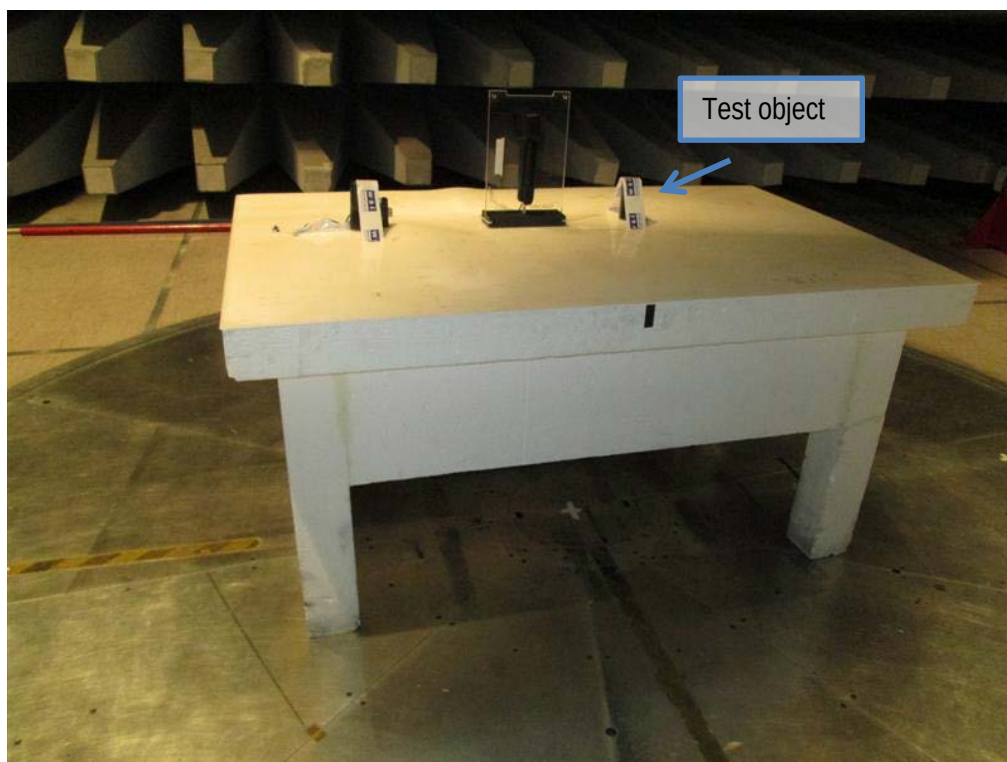
Photo 4.1.1 Test setup regarding measurement of radiated emission below 1 GHz.
