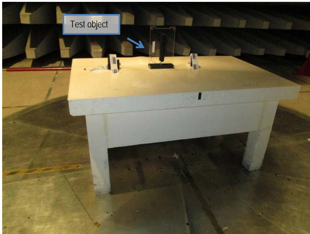
Photo 4.2.1 Test setup regarding measurement of radiated emission below 1 GHz.
