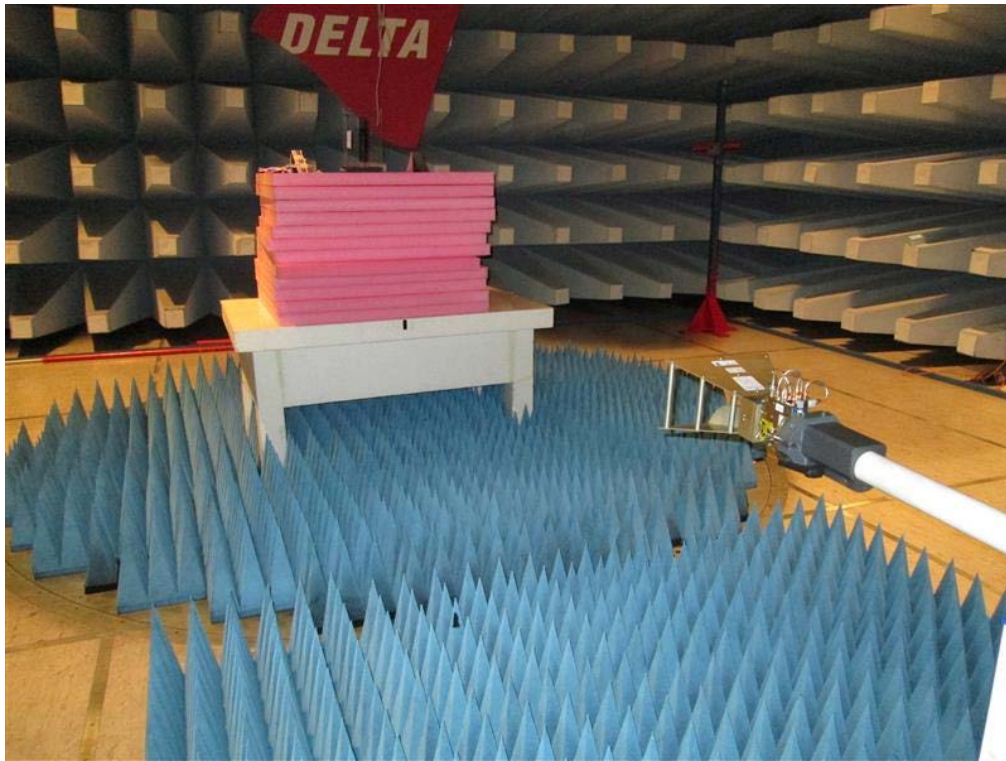
Photo 4.3.1 Test setup regarding measurement of radiated emission above 1 GHz.
