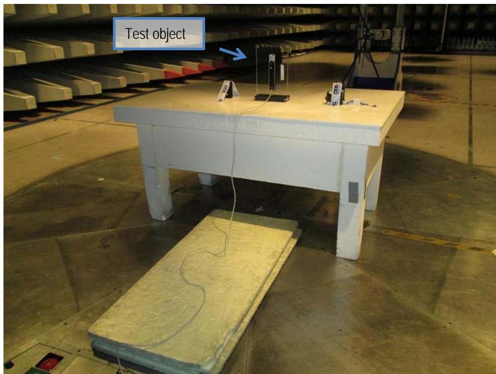
Photo 4.2.2 Test setup regarding measurement of radiated emission below 1 GHz.
