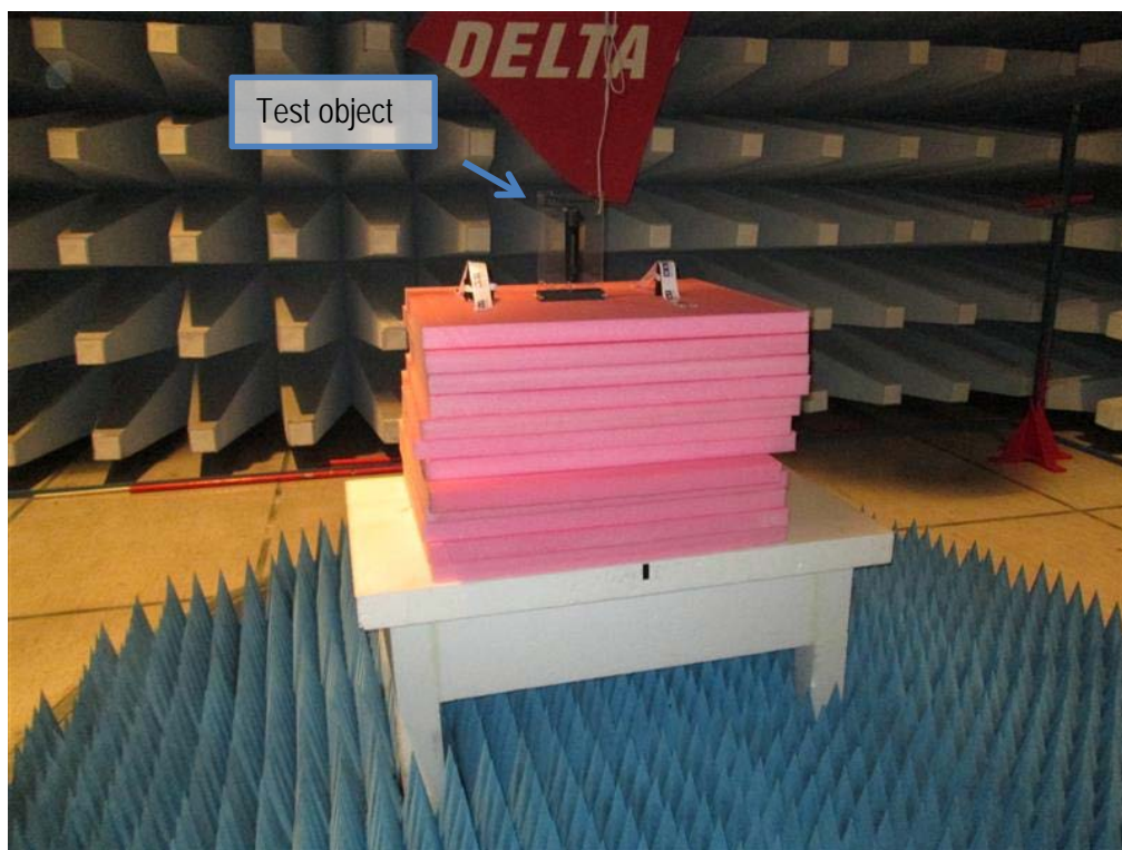
Photo 4.3.2 Test setup regarding measurement of radiated emission above 1 GHz.
