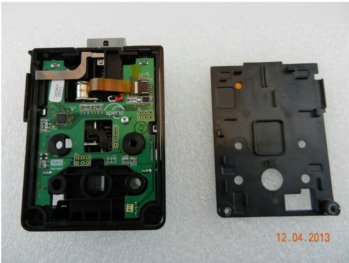
Lockbody – rear cover removed
