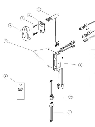
The iCLASS Module can either be supported by the electrical connection to the Electric Strike, or by mounting it directly to the back of several HES Electric Strikes using the #6-32 Module Mounting Screws. Do not attempt to support the iCLASS Module with the 18" Antenna Cable
