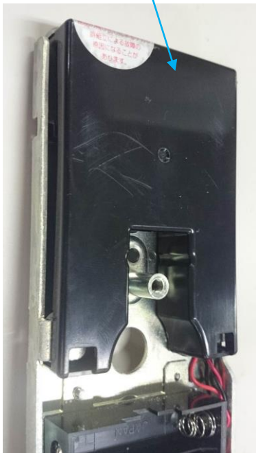
Control board resin cover
