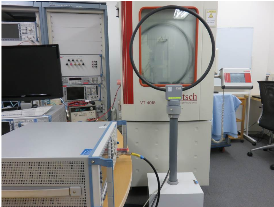
Photograph 1: Set-up for Frequency Stability, General View
