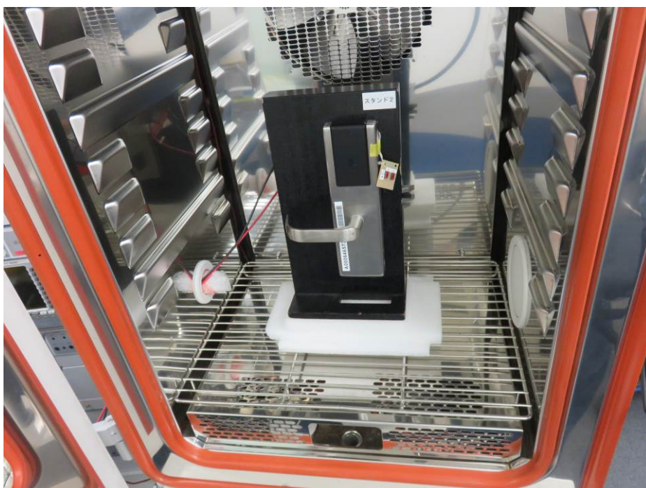
Photograph 2: Set-up for Frequency Stability, Inside Temperature Chamber
