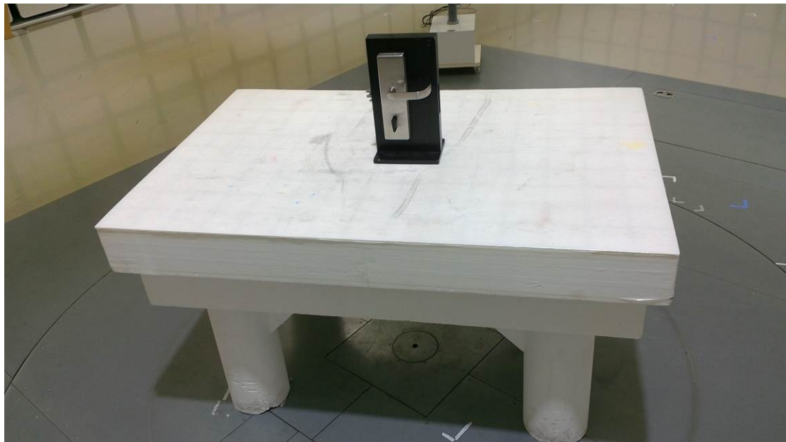
Photograph 4: Set-up for Radiated Emission of Transmitter, Rear View
