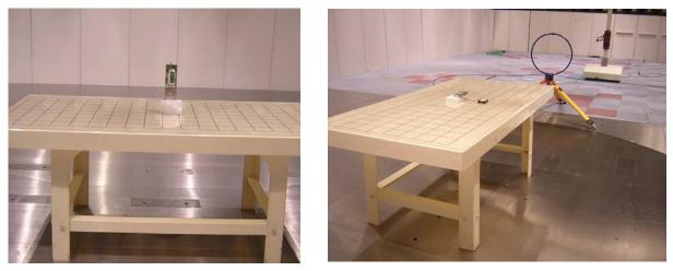
7.2 Photos of Radiated Emission Test (above 30MHz)
