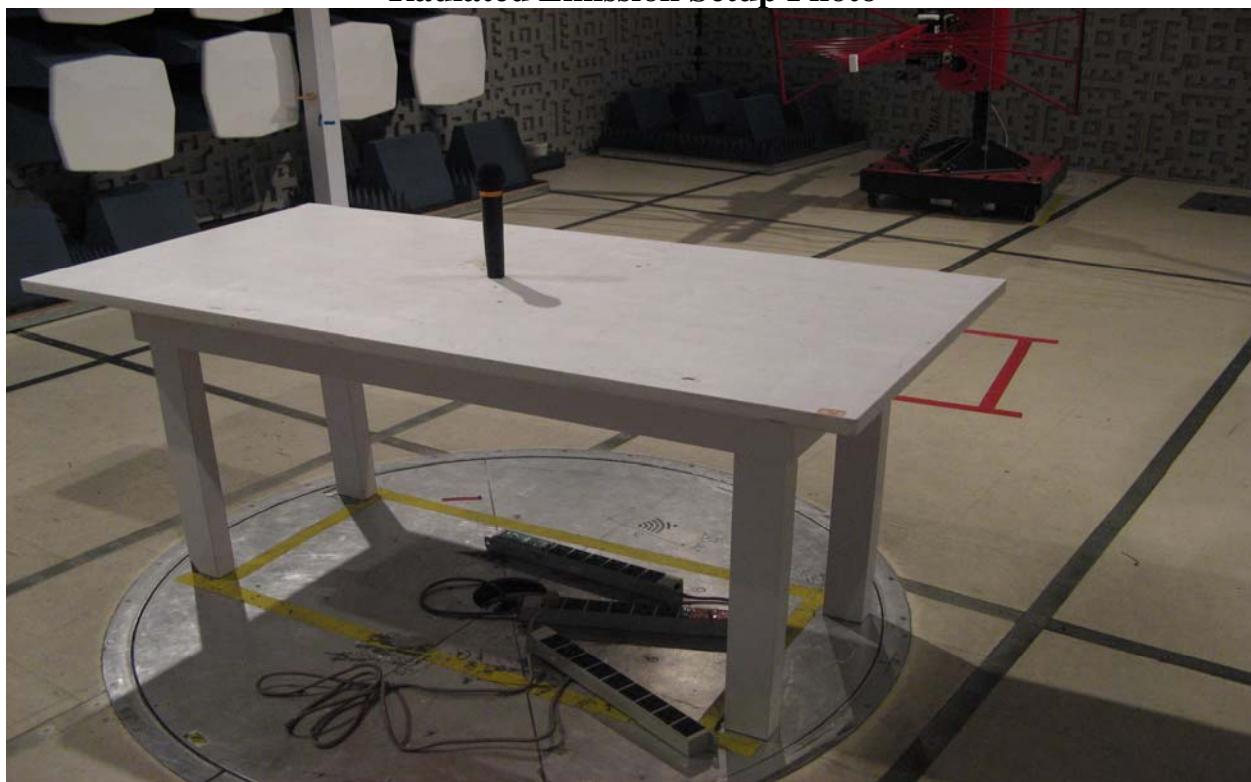
Radiated Emission Setup Photo
