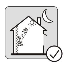
When installing outdoors, direct sunlight equipment, oblique sunlight equipment or direct sunlight equipment through window are prohibited When installing indoors, make sure that the place must be installed away from windows / doors / lamp more than 2 meters away equipment
