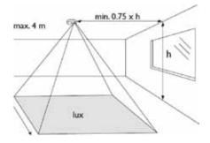
Mount multi-sensor I to .75 times window height away from the window and where the occupancy sensor can see the space to detect movement.
