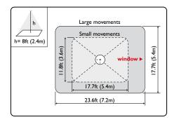
Detection area will vary based on ceiling height. For a typical ceiling height of 8 ft (2.4m): Major motion 17.7  $\times$  23.6ft (5.40m  $\times$  7.20m) Minor motion 11.8  $\times$  17.7ft (3.60m  $\times$  5.40m) Larger areas will require multiple sensors. Up to 16 device can be linked for one space. During installation the retractable sen-sor's field can be rotated to partially mask the sen-sor's field of view and prevent unwanted move-ment detection.
