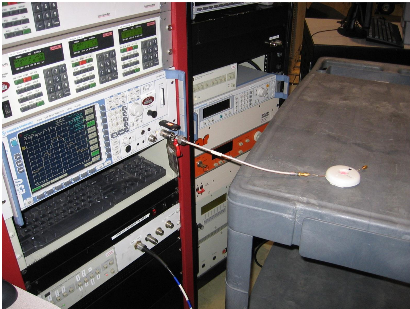
Figure 26 Test setup for Maximum Peak Output Power
