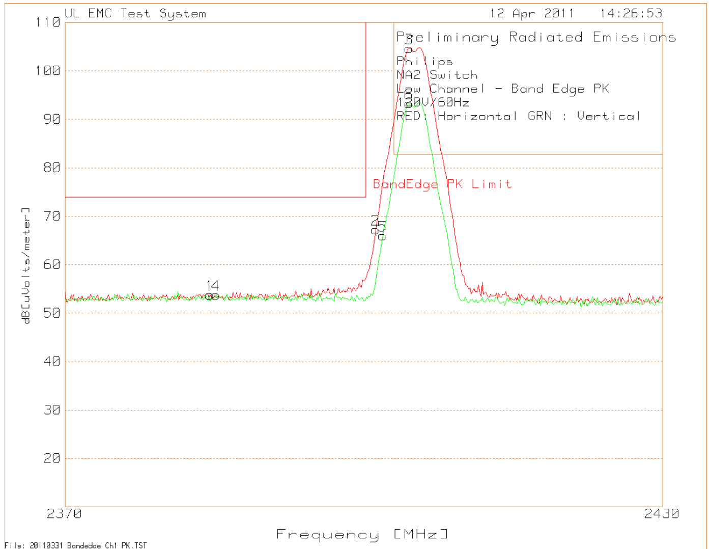
Figure 34 Radiated Band Edge Compliance Graph – Switch - Low channel - Peak
