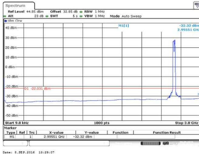
Figure 109 Spurious Emissions (9kHz – 3GHz) - QPSK (2583.0/2603.0 MHz) (2 X 20 MHz Channel BW)
