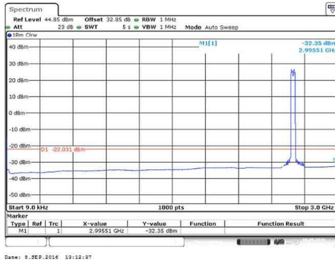
Figure 97 Spurious Emissions (9kHz – 3GHz) - QPSK (2583.0/2603.0 MHz) (2 X 20 MHz Channel BW)
