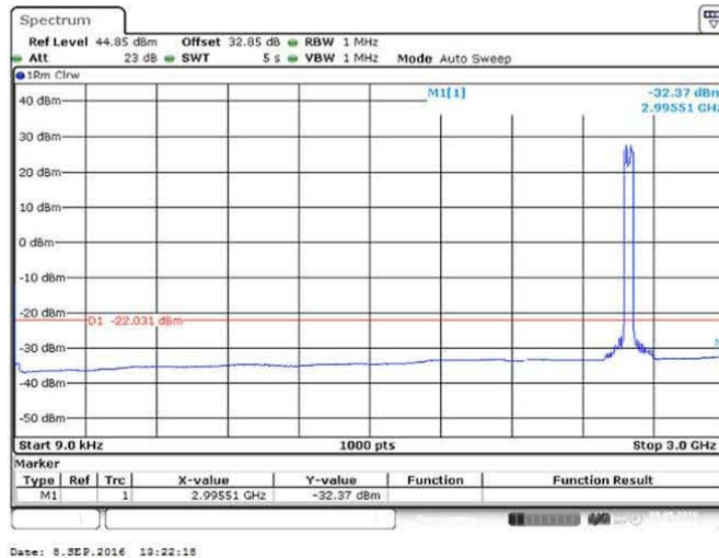
Figure 105 Spurious Emissions (9kHz – 3GHz) – 16QAM (2583.0/2603.0 MHz) (2 X 20 MHz Channel BW)
