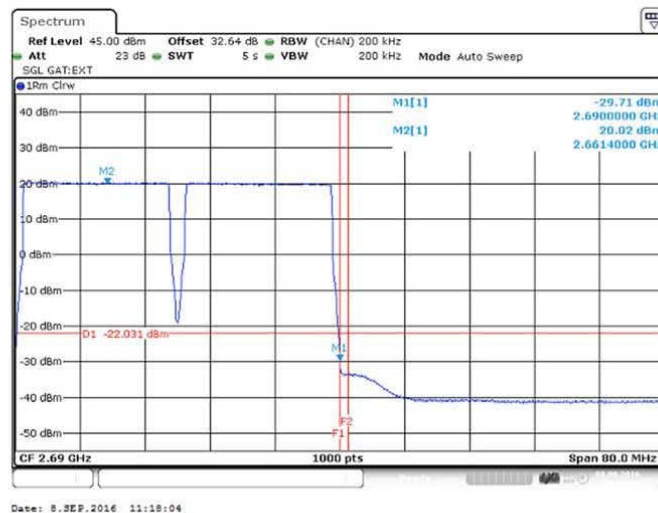
Figure 148 Spurious Emissions (Upper Band Edge) – 64QAM (2660.0/2680.0 MHz) (2 X 20 MHz Channel BW)
