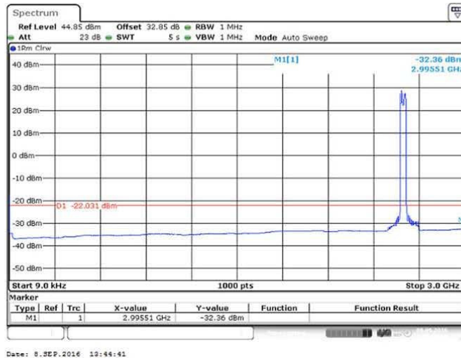
Figure 117 Spurious Emissions (9kHz – 3GHz) – 16QAM (2583.0/2603.0 MHz) (2 X 20 MHz Channel BW)
