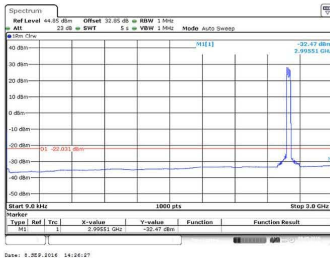
Figure 145 Spurious Emissions (9kHz – 3GHz) – QPSK (2583.0/2603.0 MHz) (2 X 20 MHz Channel BW)
