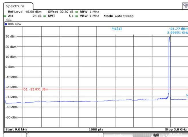
Figure 140 Spurious Emissions (9kHz – 3GHz) – 16QAM (2593.0 MHz) (20MHz Channel BW)
