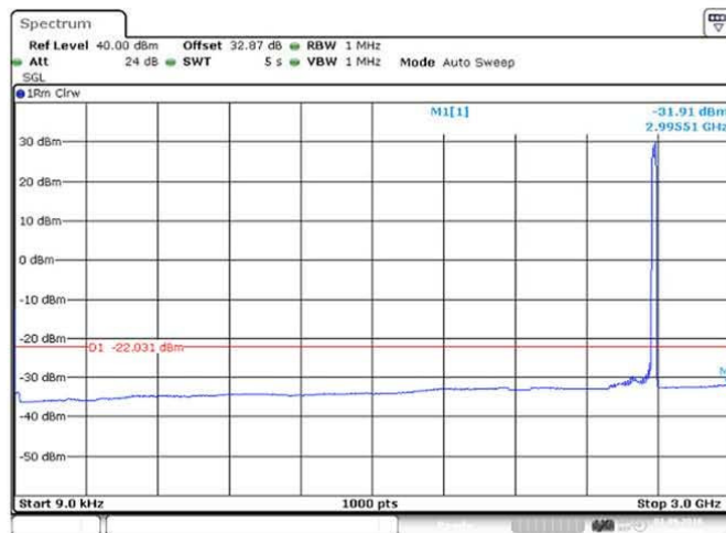
Figure 65 Spurious Emissions (9kHz – 3GHz) – 64QAM (2593.0 MHz) (20MHz Channel BW)
