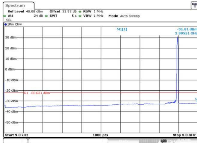
Figure 57 Spurious Emissions (9kHz – 3GHz) – 16QAM (2593.0 MHz) (20MHz Channel BW)
