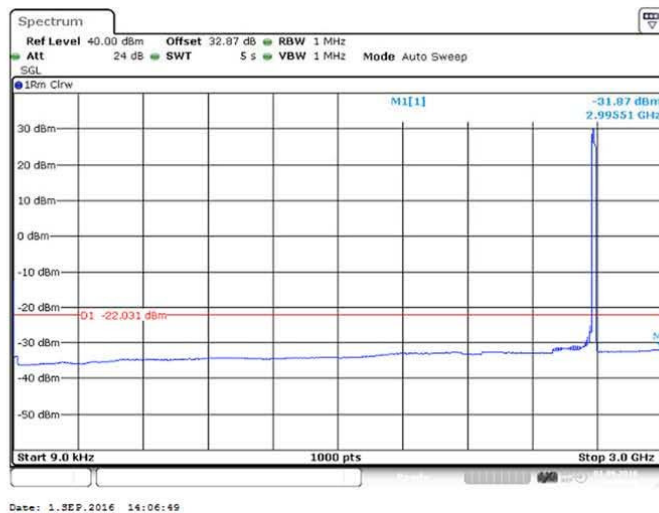
Figure 144 Spurious Emissions (9kHz – 3GHz) – QPSK (2593.0 MHz) (20MHz Channel BW)
