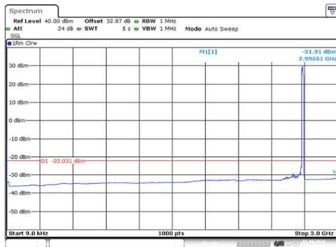
Figure 69 Spurious Emissions (9kHz – 3GHz) – 16QAM (2593.0 MHz) (20MHz Channel BW)
