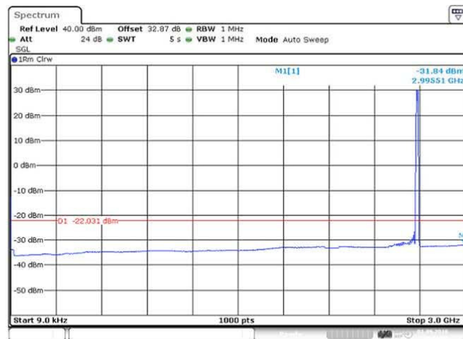
Figure 53 Spurious Emissions (9kHz – 3GHz) – 64QAM (2593.0 MHz) (20MHz Channel BW)
