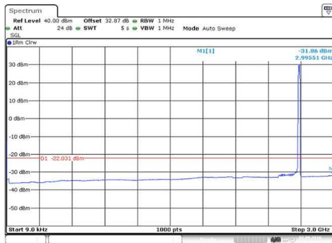
Figure 132 Spurious Emissions (9kHz – 3GHz) - QPSK (2593.0 MHz) (20MHz Channel BW)
