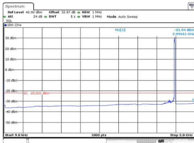
Figure 125 Spurious Emissions (9kHz – 3GHz) – 64QAM (2593.0 MHz) (20MHz Channel BW)
