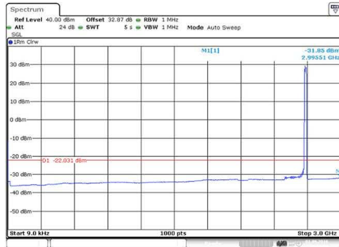
Figure 45 Spurious Emissions (9kHz – 3GHz) – 16QAM (2593.0 MHz) (20MHz Channel BW)
