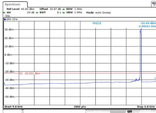
Figure 121 Spurious Emissions (9kHz – 3GHz) - QPSK (2593.0 MHz) (20MHz Channel BW)
