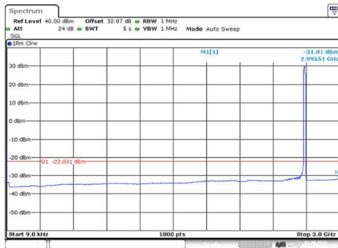
Figure 117 Spurious Emissions (9kHz – 3GHz) – 16QAM (2593.0 MHz) (20MHz Channel BW)
