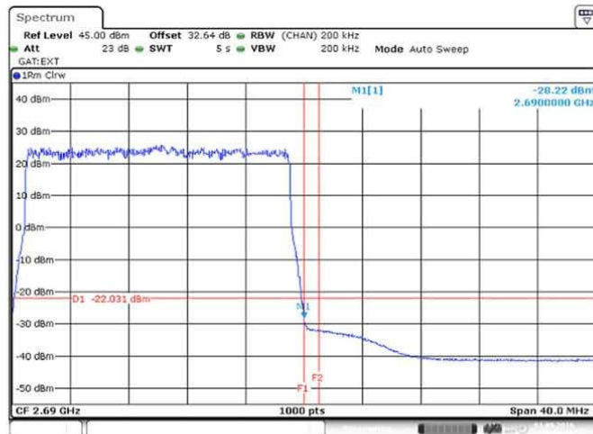
Figure 116 Spurious Emissions (Upper Band Edge) – 16QAM (2680.0 MHz) (20MHz Channel BW)
