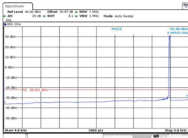
Figure 109 Spurious Emissions (9kHz – 3GHz) - QPSK (2593.0 MHz) (20MHz Channel BW)
