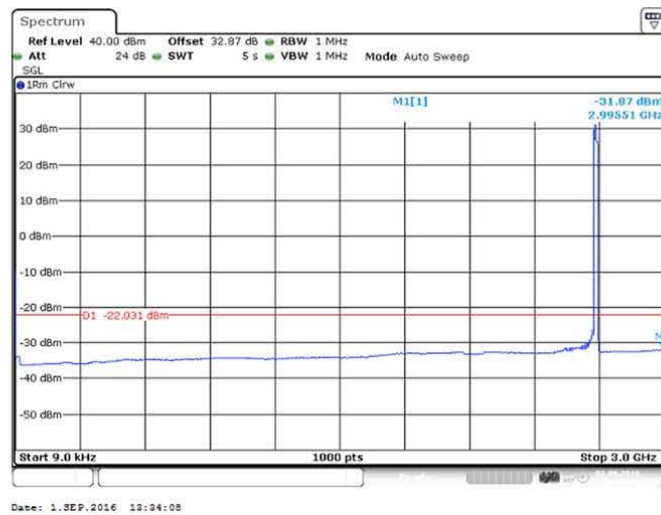
Figure 113 Spurious Emissions (9kHz – 3GHz) – 64QAM (2593.0 MHz) (20MHz Channel BW)
