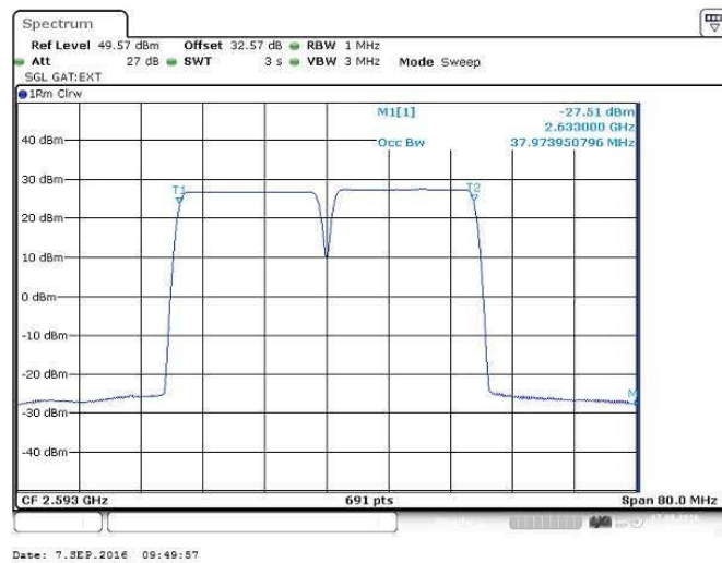
Figure 44 Occupied Bandwidth –QPSK (2583/ 2603 MHz) (2 X 20MHz Channel BW)
