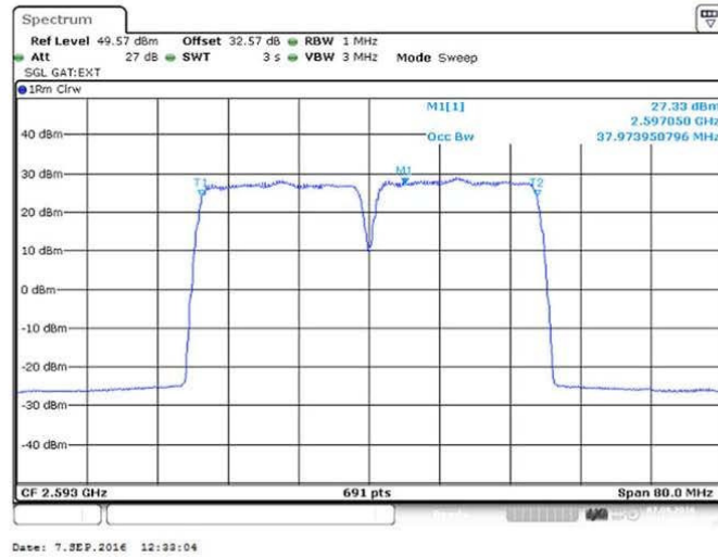
Figure 58 Occupied Bandwidth –16QAM (2583/ 2603 MHz) (2 X 20 MHz Channel BW)
