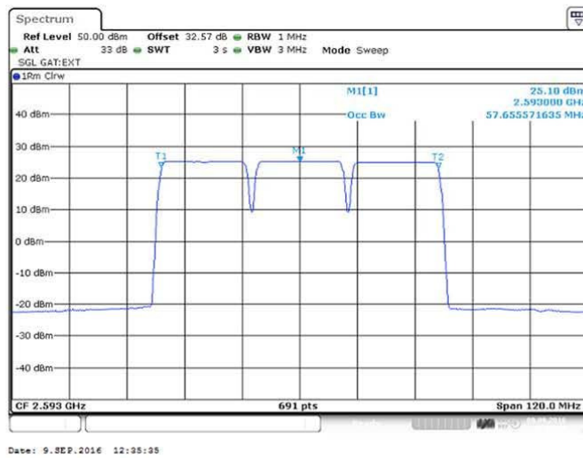
Figure 77 Occupied Bandwidth –QPSK (2573/ 2593/ 2613 MHz) (3 X 20 MHz Channel BW)
