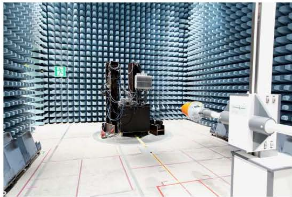
Figure 38870 Photograph of the anechoic chamber with the EUT
