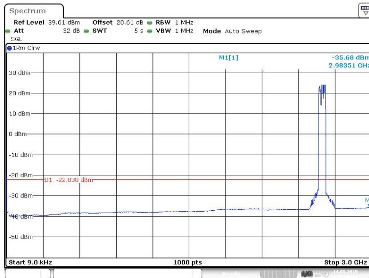
Figure 366 Spurious Emissions (9kHz – 3GHz) - QPSK (2573.0/2593.0/2613 MHz) (20MHz Channel BW)
