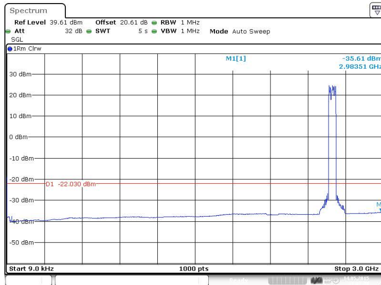
Figure 382 Spurious Emissions (9kHz – 3GHz) - 16QAM (2573.0/2593.0/2613 MHz) (20MHz Channel BW)
