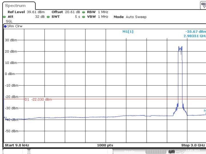
Figure 378 Spurious Emissions (9kHz – 3GHz) - QPSK (2573.0/2593.0/2613 MHz) (20MHz Channel BW)
