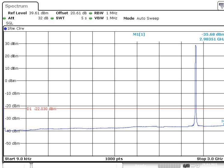
Figure 43 Spurious Emissions (9kHz – 3GHz) – QPSK (2593.0 MHz) (15MHz Channel BW)
