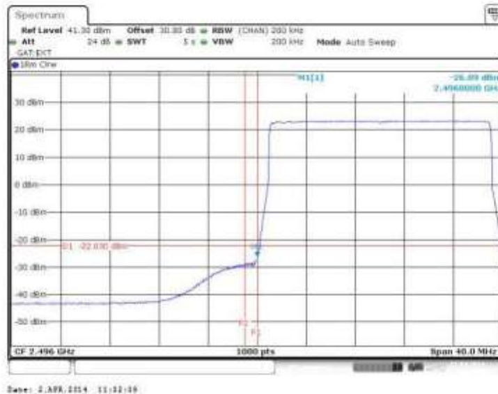
Figure 91 Spurious Emissions (Lower Band Edge) – 64QAM (2506.0 MHz) (20MHz Channel BW)
