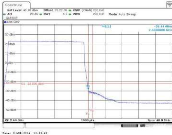
Figure 116 Spurious Emissions (Upper Band Edge) – 64QAM (2680.0 MHz) (20MHz Channel BW)
