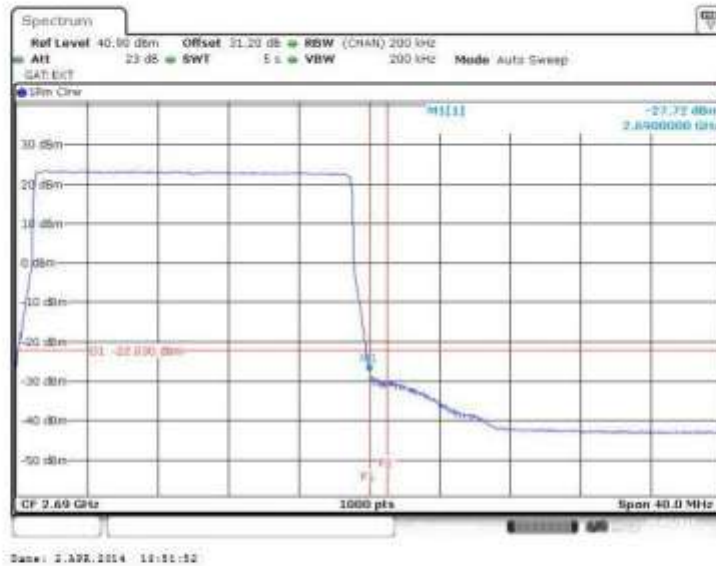
Figure 128 Spurious Emissions (Upper Band Edge) – 64QAM (2680.0 MHz) (20MHz Channel BW)
