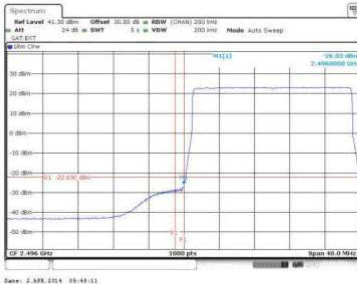
Figure 79 Spurious Emissions (Lower Band Edge) – 64QAM (2506.0 MHz) (20MHz Channel BW)
