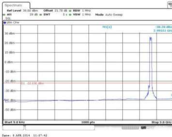
Figure 141 Spurious Emissions (9kHz – 3GHz) – 64QAM (2583.0/2603.0 MHz) (20MHz Channel BW)
