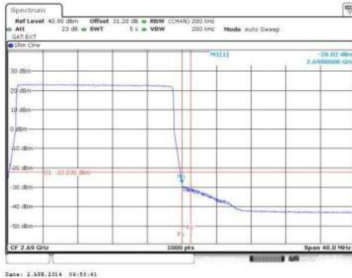
Figure 80 Spurious Emissions (Upper Band Edge) – 64QAM (2680.0 MHz) (20MHz Channel BW)
