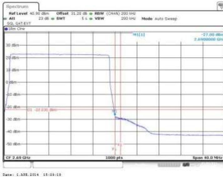
Figure 44 Spurious Emissions (Upper Band Edge) – 64QAM (2680.0 MHz) (20MHz Channel BW)
