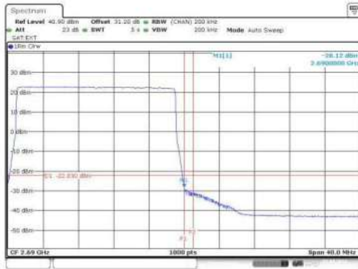
Figure 68 Spurious Emissions (Upper Band Edge) – 64QAM (2680.0 MHz) (20MHz Channel BW)
