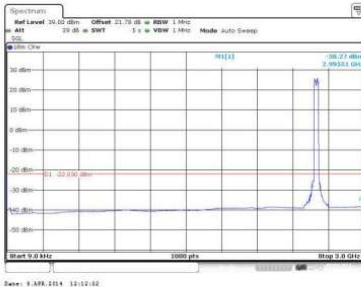
Figure 157 Spurious Emissions (9kHz – 3GHz) - QPSK (2583.0/2603.0 MHz) (20MHz Channel BW)
