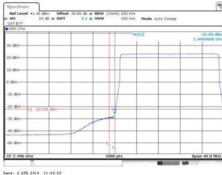
Figure 55 Spurious Emissions (Lower Band Edge) – 64QAM (2506.0 MHz) (20MHz Channel BW)
