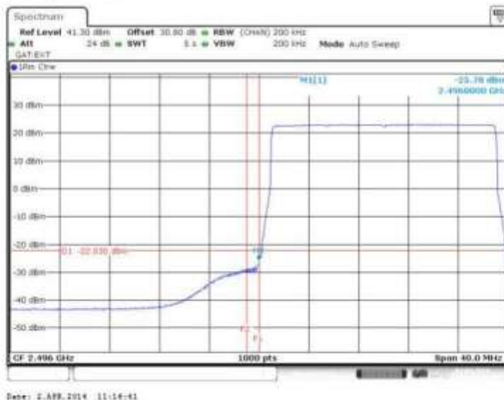
Figure 83 Spurious Emissions (Lower Band Edge) – QPSK (2506.0 MHz) (20MHz Channel BW)
