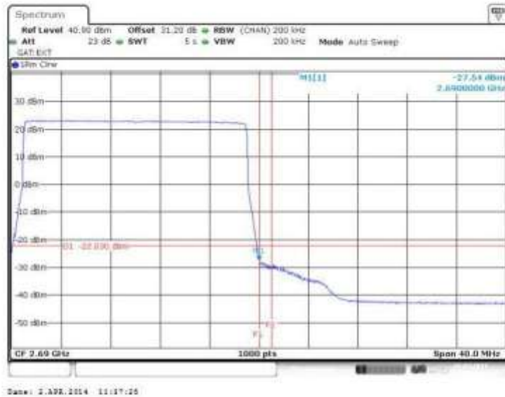
Figure 92 Spurious Emissions (Upper Band Edge) – 64QAM (2680.0 MHz) (20MHz Channel BW)
