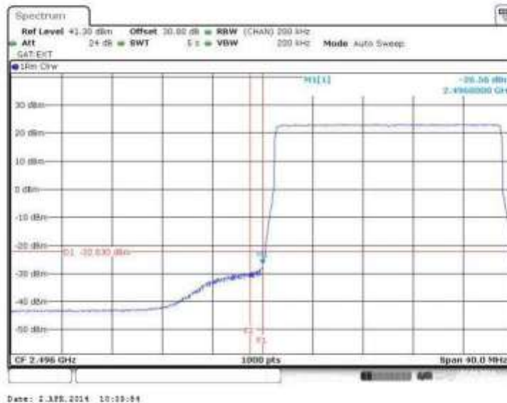
Figure 67 Spurious Emissions (Lower Band Edge) – 64QAM (2506.0 MHz) (20MHz Channel BW)
