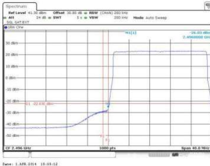
Figure 43 Spurious Emissions (Lower Band Edge) – 64QAM (2506.0 MHz) (20MHz Channel BW)
