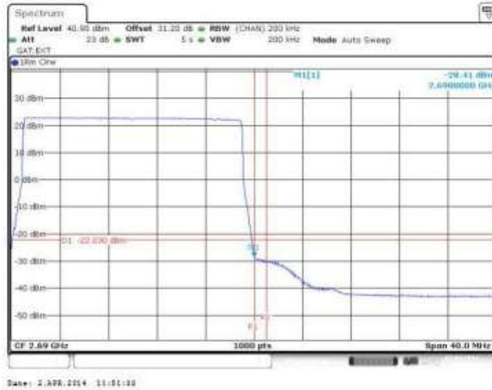
Figure 96 Spurious Emissions (Upper Band Edge) – QPSK (2680.0 MHz) (20MHz Channel BW)
