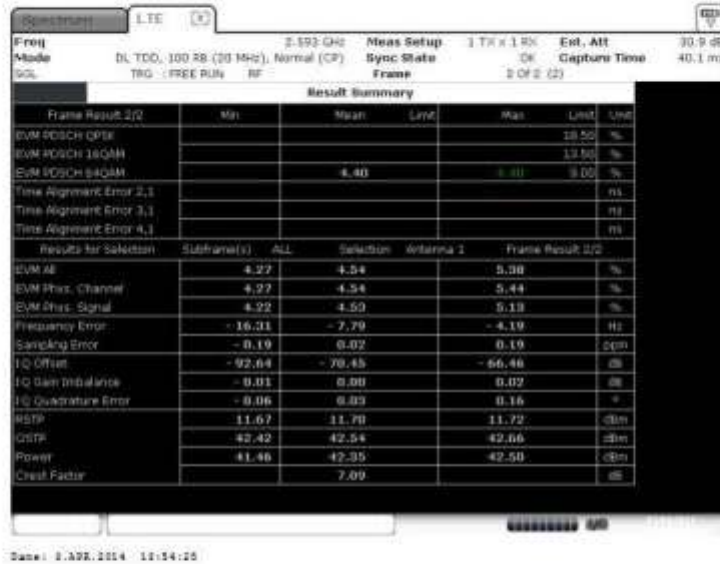
Figure 10 I/Q constellation table with I/Q error – 64QAM (2593.0 MHz) (20MHz Channel BW)
