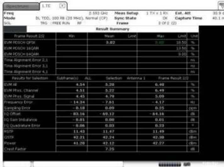
Figure 6 I/Q constellation table with I/Q error – QPSK (2593.0 MHz) (20MHz Channel BW)
