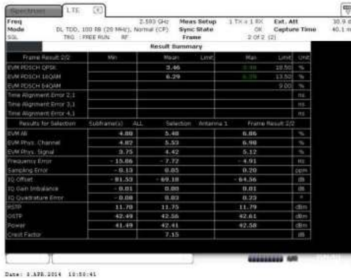
Figure 8 I/Q constellation table with I/Q error – 16QAM (2593.0 MHz) (20MHz Channel BW)
