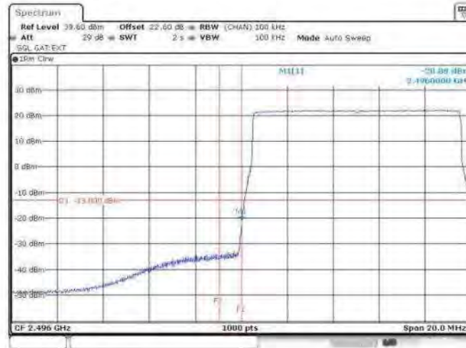
Figure 65 Spurious Emissions (Lower Band Edge) – QPSK (2501.0 MHz) (10MHz Channel BW)
