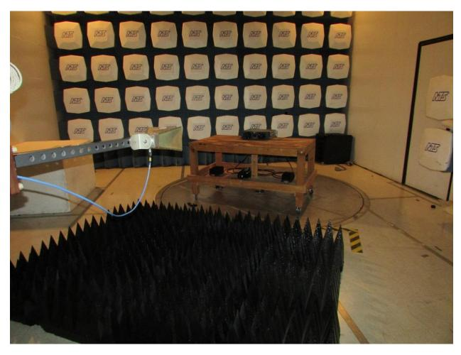
1-18GHz Radiated Measurements
