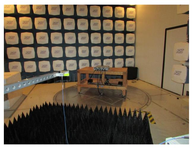
18-20GHz Radiated Measurements
