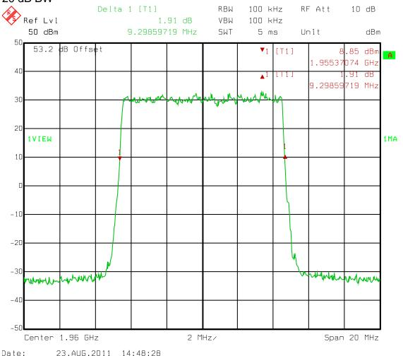
Test Data – Occupied Bandwidth 10 MHz Channel 64 QAM Center Channel 20 dB BW
