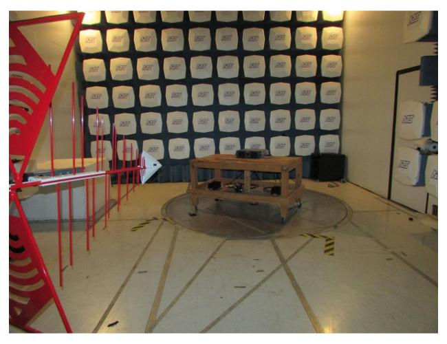
30-1000MHz Radiated Measurements
