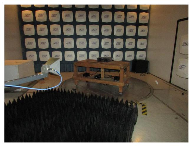
1-10GHz Radiated Measurements
