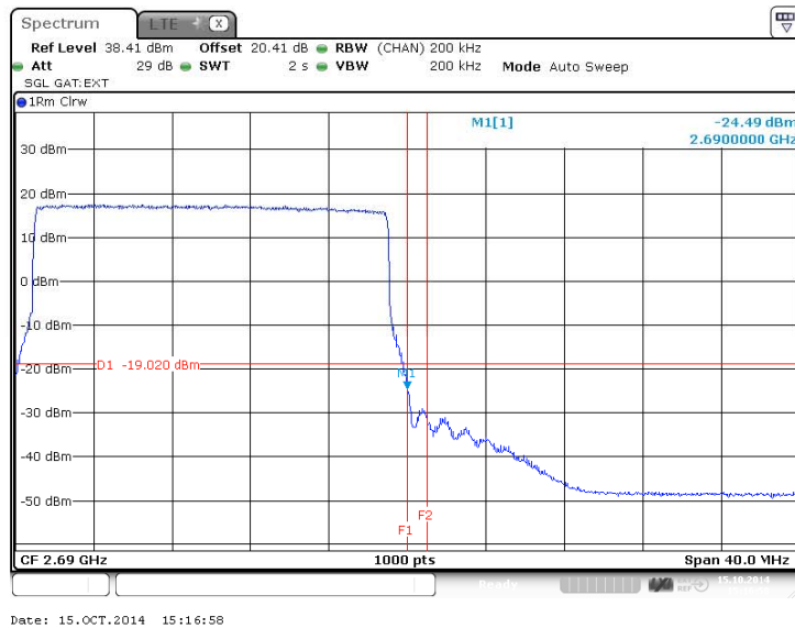
Figure 224 Spurious Emissions (Upper Band Edge) – 64QAM (2680.0 MHz) (20MHz Channel BW)
