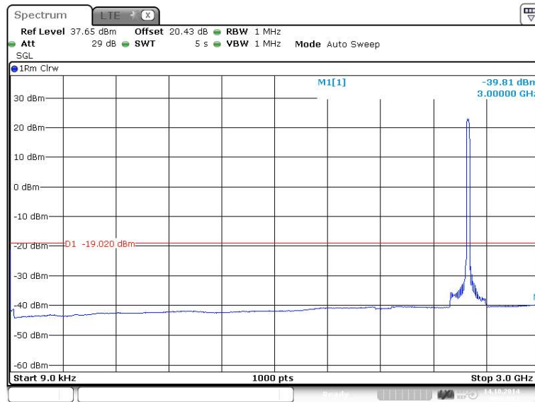
Figure 229 Spurious Emissions (9kHz – 3GHz) - QPSK (2593.0 MHz) (20MHz Channel BW)
