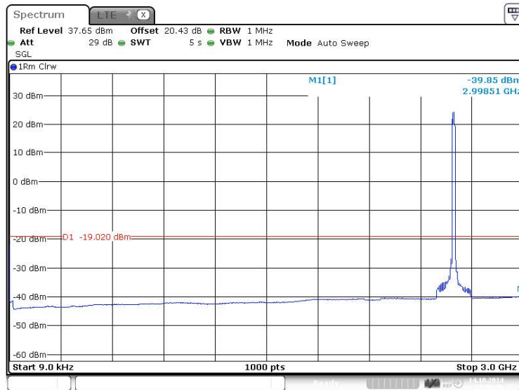
Figure 213 Spurious Emissions (9kHz – 3GHz) – 64QAM (2593.0 MHz) (20MHz Channel BW)
