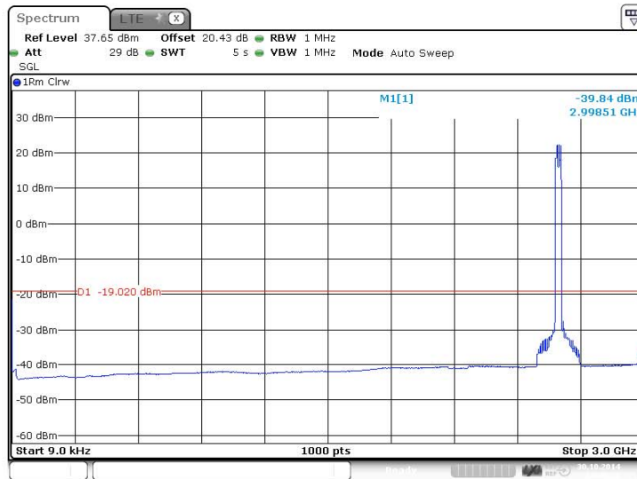
Figure 181 Spurious Emissions (9kHz – 3GHz) - QPSK (2585.5/2600.5 MHz) (15MHz Channel BW)
