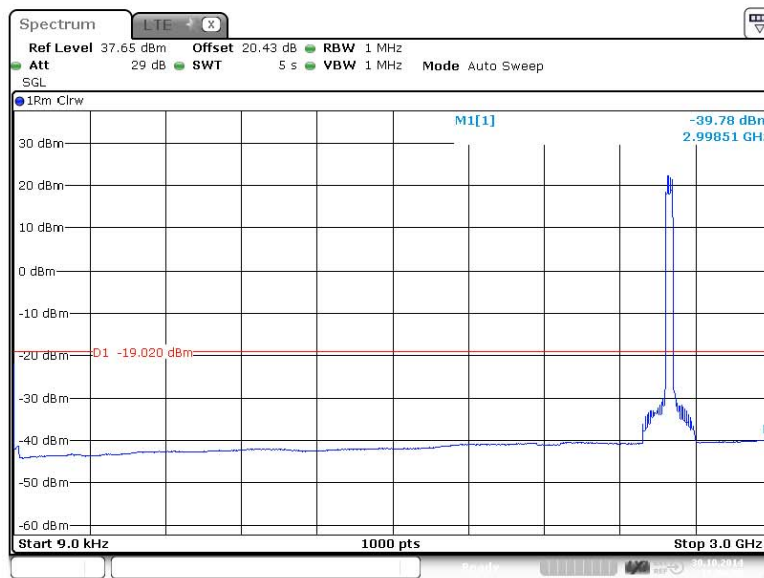
Figure 189 Spurious Emissions (9kHz – 3GHz) – 64QAM (2585.5/2600.5 MHz) (15MHz Channel BW)
