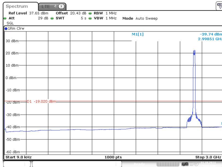
Figure 177 Spurious Emissions (9kHz – 3GHz) – 64QAM (2585.5/2600.5 MHz) (15MHz Channel BW)
