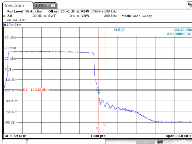
Figure 163 Spurious Emissions (Lower Band Edge) – 64QAM (2503.5 MHz) (10MHz Channel BW)
