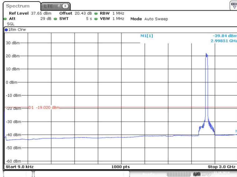
Figure 169 Spurious Emissions (9kHz – 3GHz) - QPSK (2585.5/2600.5 MHz) (15MHz Channel BW)
