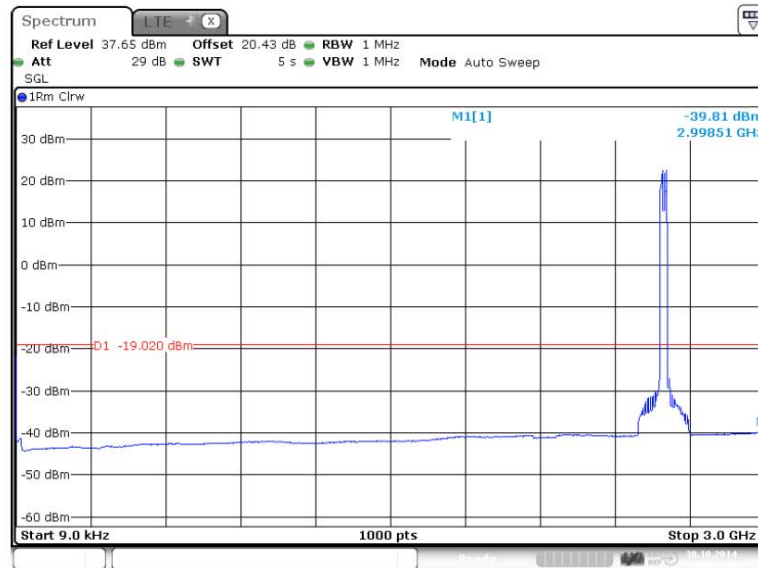
Figure 185 Spurious Emissions (9kHz – 3GHz) – 16QAM (2585.5/2600.5 MHz) (15MHz Channel BW)
