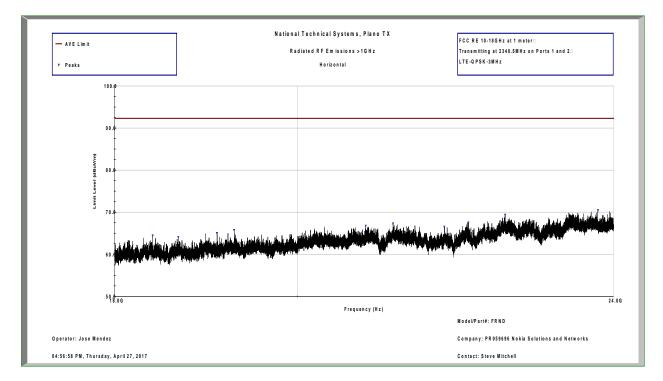
18GHz – 24GHz Peak Prescan at 3m – V
