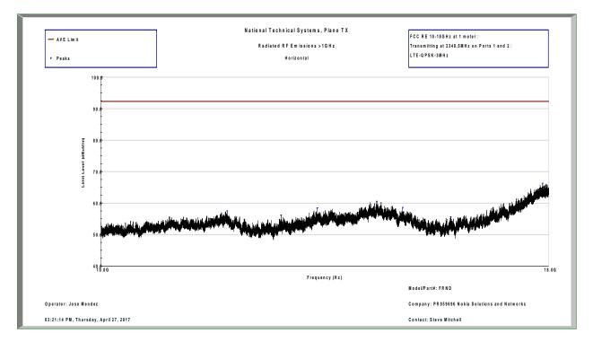
10GHz – 18GHz Peak Prescan at 3m – V
