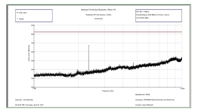
1GHz – 10GHz Peak Prescan at 3m – V
