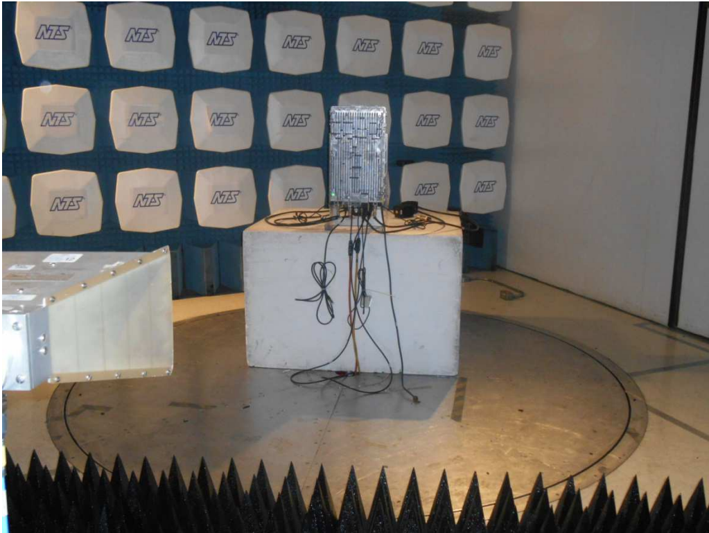
Radiated Emissions Setup – 1GHz to 18GHz
