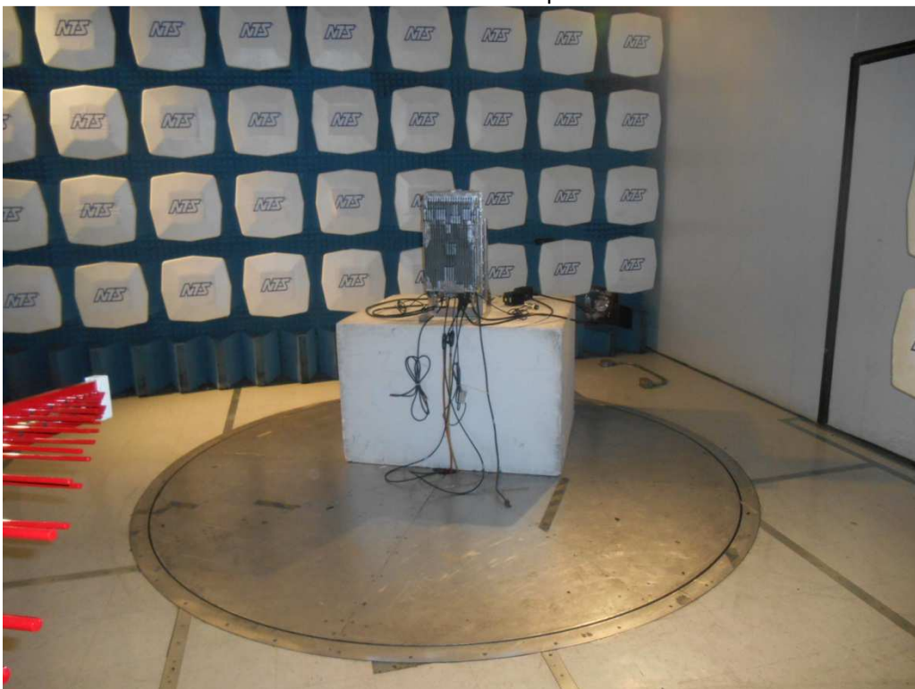
Radiated Emissions Setup – 30MHz to 1GHz
