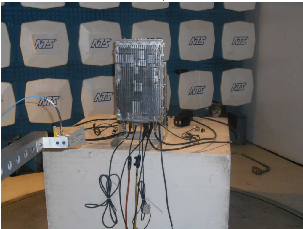
Radiated Emissions Setup – 18GHz to 24GHz
