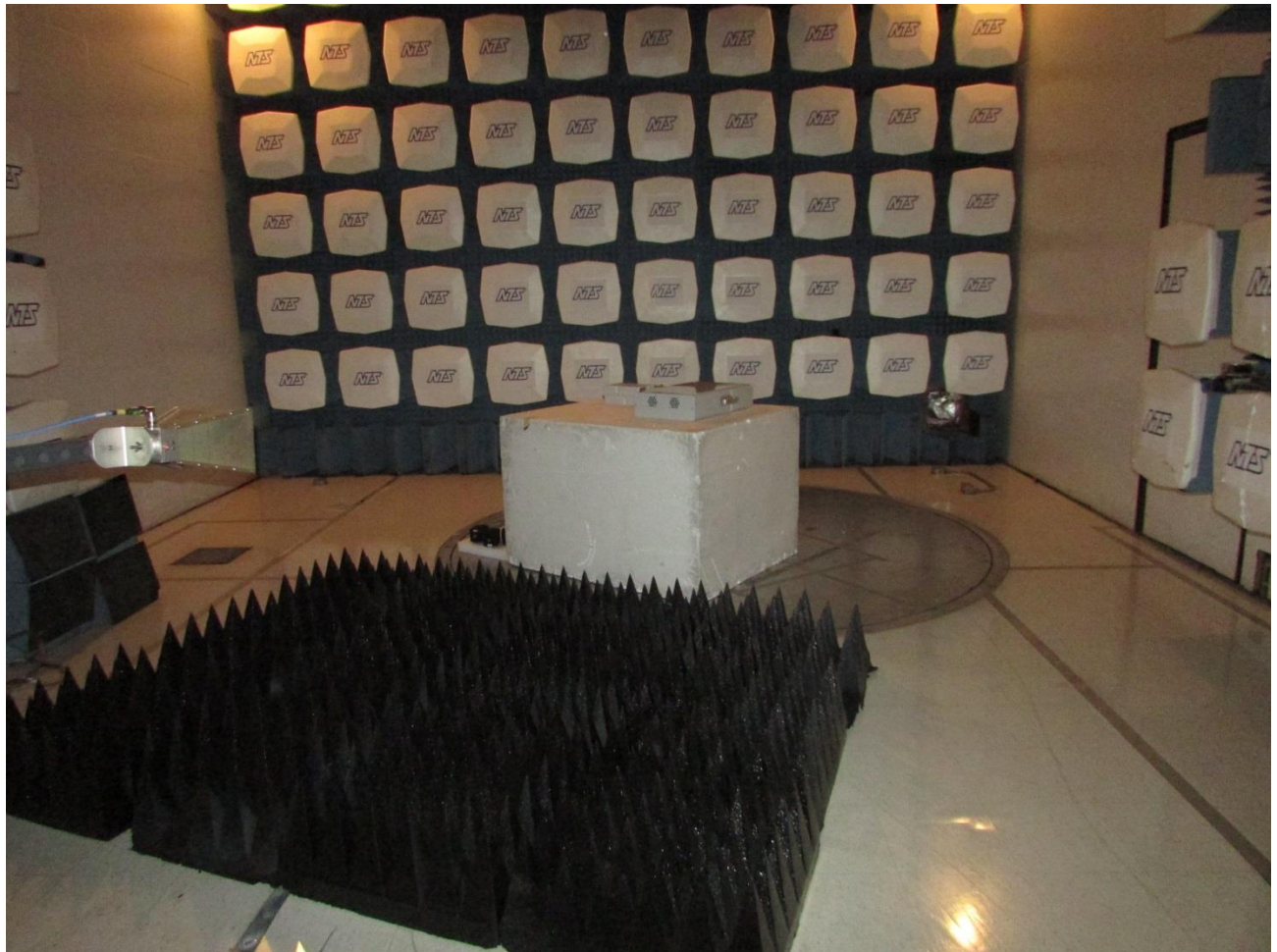
AWS - 4 Band Out of Band Radiated Emissions test setup
