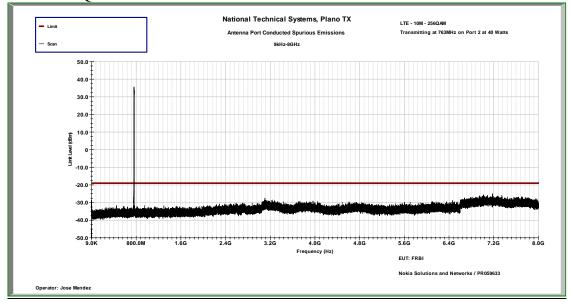
The FCC section 90.543(e)(1) requires an emission limit of -46dBm for any 6.25 kHz bandwidth (i.e.: 76 + 10logP) between frequency bands 769-775 MHz and 799-805 MHz. Adjusting for the required measurement RBW and four port MIMO requirement the emission limit in these frequency ranges is -40 dBm [i.e.: Limit = -46 dBm/6.25kHz (FCC Limit) + 12dB (BW conversion 10 log [100kHz/6.25kHz]) – 6dB (4 port MIMO)].
