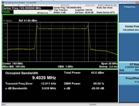
Channel Frequency 740 MHz, Modulation QPSK, TX1
