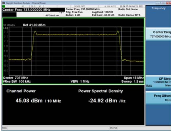
Channel Frequency 737 MHz, Modulation QPSK, TX1
