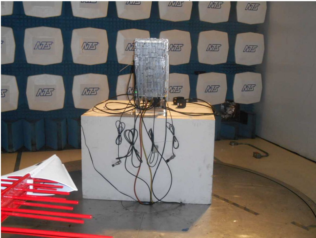
Radiated Emissions Setup – 30MHz to 1GHz
