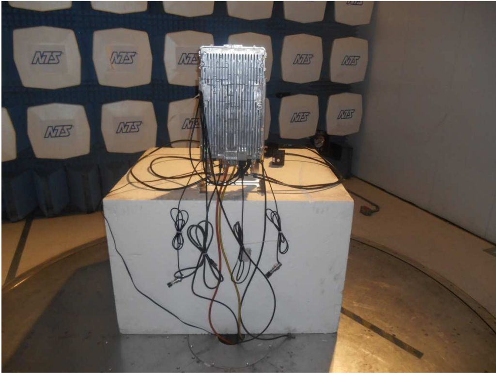
Radiated Emissions Setup - Front
