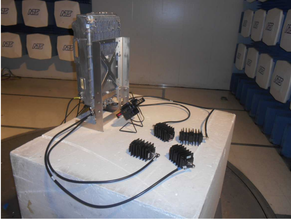
Radiated Emissions Setup – Rear
