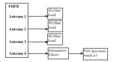
Test Setup Used for FHFB Conducted RF Measurements
