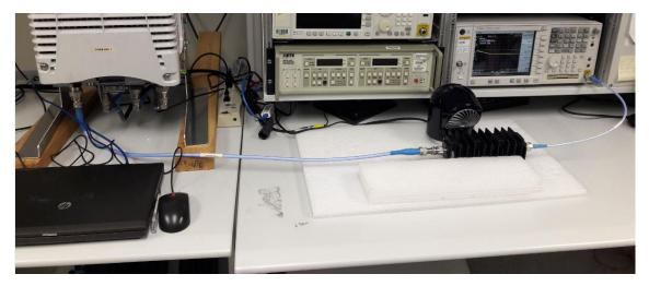
Photograph of 20MHz to 3GHz and 3GHz to 6GHz Test Setup
