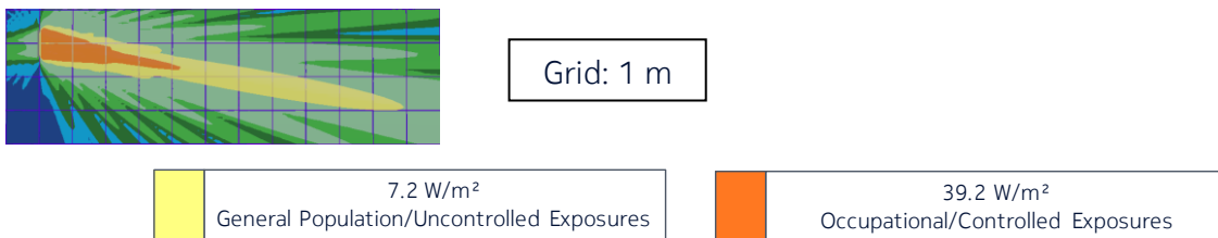
Figure 13 – Side view of the power density for the time-averaged actual maximum transmitted power of 85 W and the beam oriented in azimuth = 0° & elevation = +10° (Canada)
