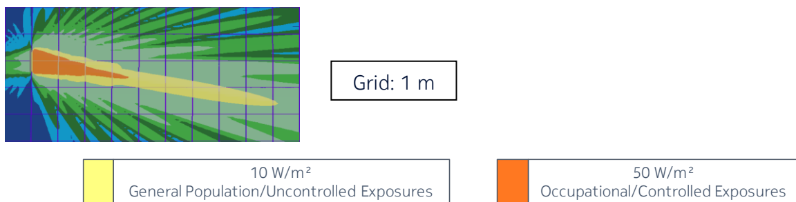
Figure 5 – Side view of the power density for the time-averaged actual maximum transmitted power of 85 W and the beam oriented in azimuth = 0° & elevation = +10° (EU/ICNIRP, Australia/NZ and US/related)
