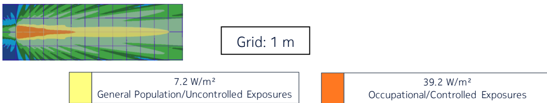
Figure 15 – Side view of the power density for the time-averaged actual maximum transmitted power of 85 W and the beam oriented in azimuth = 0° & elevation = 0° (Canada)
