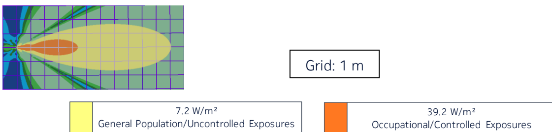
Figure 11 – Top view of the power density for the time-averaged actual maximum transmitted power of 85 W and the beam oriented in azimuth = 0° & elevation = 0° (Canada)
