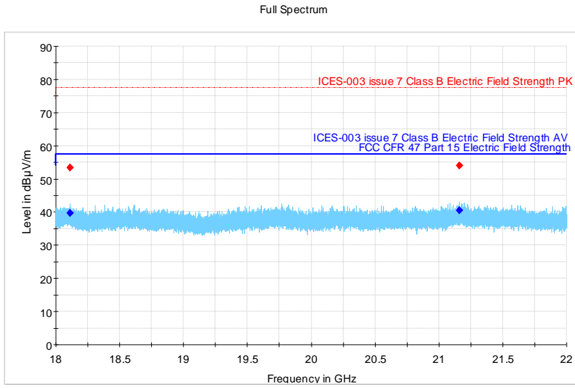
Figure 20 Field Strength of Spurious Radiation (18 GHz – 22 GHz) – QPSK (1940 / 1985 / 2120 / 2190 MHz) (20+20+20+20 MHz Channel BW)
