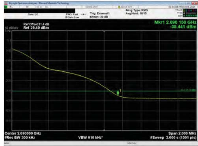
Port 1 30 MHz Channel Bandwidth QPSK Modulation High Channel, 2674.98 MHz 2689.0 MHz - 2691.0 MHz
