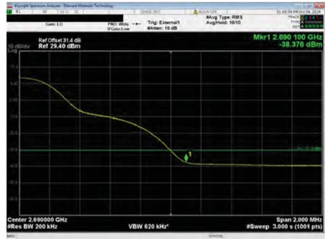
Port 1 20 MHz Channel Bandwidth QPSK Modulation High Channel, 2679.99 MHz 2689.0 MHz - 2691.0 MHz
