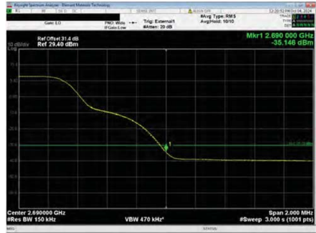
Port 1 15 MHz Channel Bandwidth QPSK Modulation High Channel, 2682.48 MHz 2689.0 MHz - 2691.0 MHz
