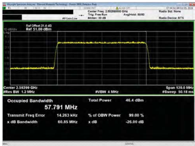
Port 1 60 MHz Channel Bandwidth 64QAM Modulation Mid Channel, 2592.99 MHz
