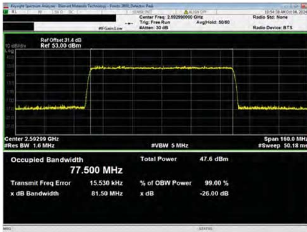
Port 1 80 MHz Channel Bandwidth 64QAM Modulation Mid Channel, 2592.99 MHz
