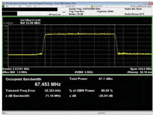
Port 1 70 MHz Channel Bandwidth QPSK Modulation Low Ch, 2531.01 MHz
