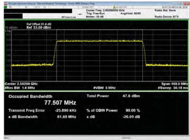
Port 1 80 MHz Channel Bandwidth 256QAM Modulation Mid Channel, 2592.99 MHz
