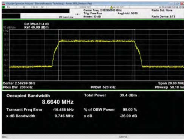
Port 1 10 MHz Channel Bandwidth 64QAM Modulation Mid Channel, 2592.99 MHz
