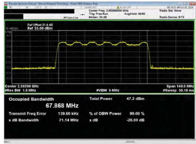
Port 1 70 MHz Channel Bandwidth 16QAM Modulation Mid Channel, 2592.99 MHz
