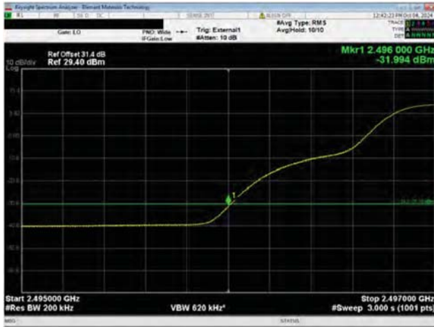
Port 1 20 MHz Channel Bandwidth QPSK Modulation Low Channel, 2506.02 MHz 2495.0 MHz - 2497.0 MHz
