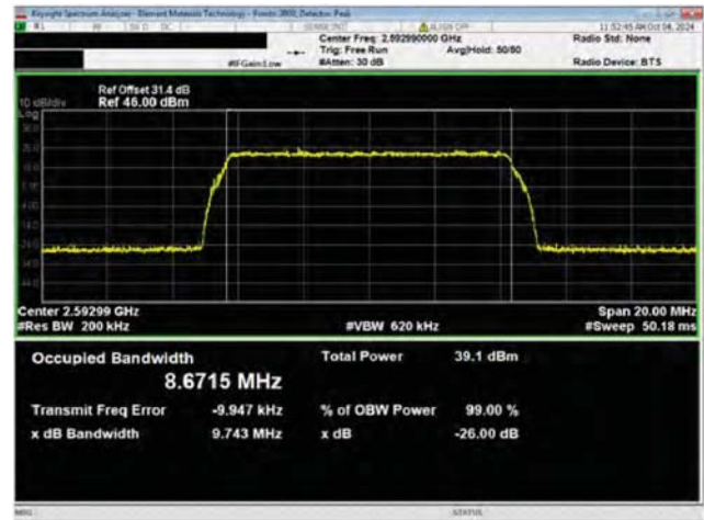
Port 1 10 MHz Channel Bandwidth 256QAM Modulation Mid Channel, 2592.99 MHz
