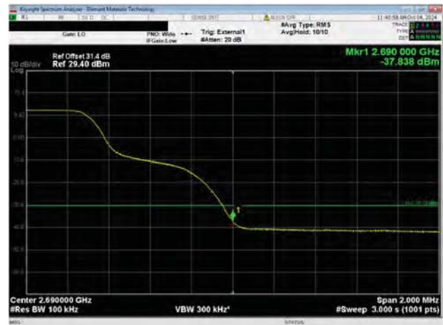
Port 1 10 MHz Channel Bandwidth QPSK Modulation High Channel, 2685.00 MHz 2689.0 MHz - 2691.0 MHz
