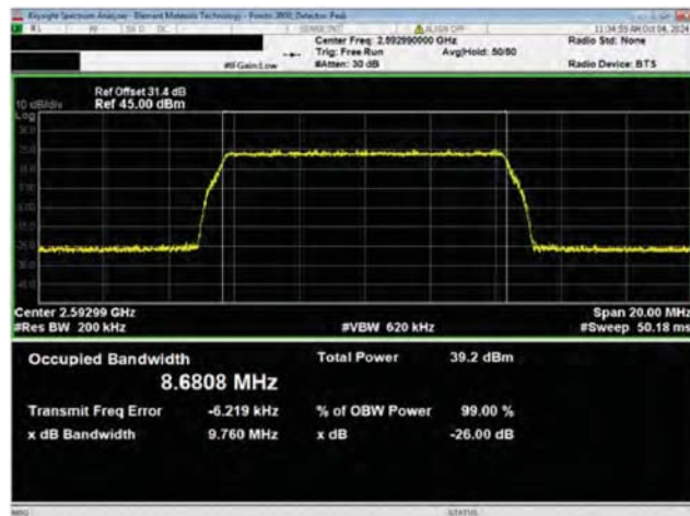
Port 1 10 MHz Channel Bandwidth QPSK Modulation Mid Channel, 2592.99 MHz
