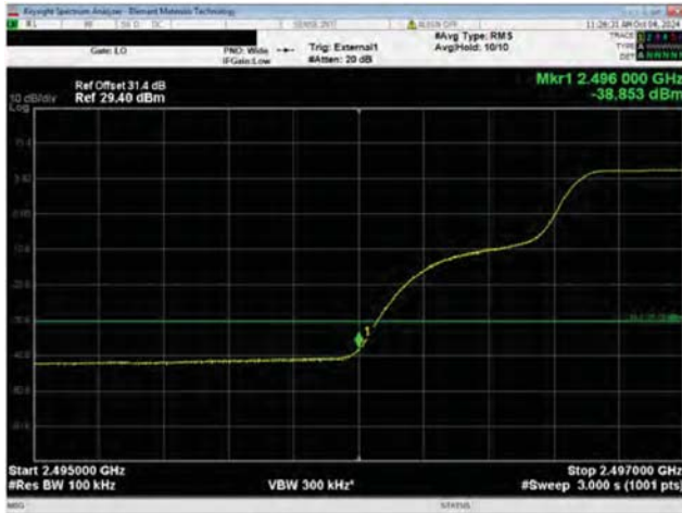
Port 1 10 MHz Channel Bandwidth QPSK Modulation Low Channel, 2501.01 MHz 2495.0 MHz - 2497.0 MHz
