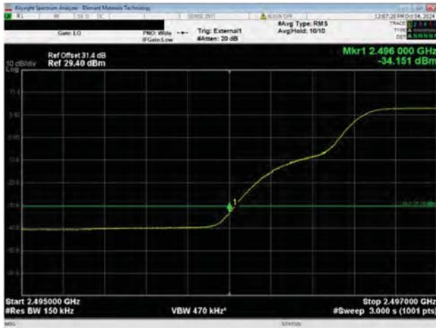
Port 1 15 MHz Channel Bandwidth QPSK Modulation Low Channel, 2503.50 MHz 2495.0 MHz - 2497.0 MHz
