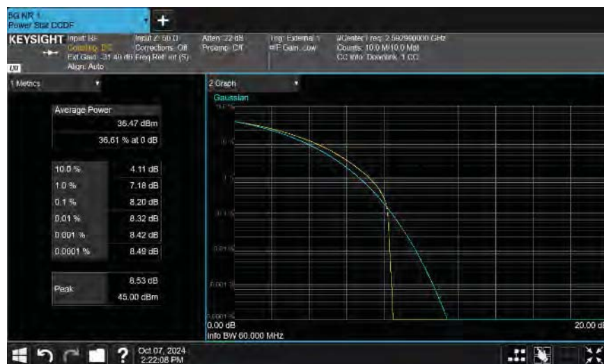
Port 1 60 MHz Channel Bandwidth QPSK Modulation Mid Channel, 2592.99 MHz
