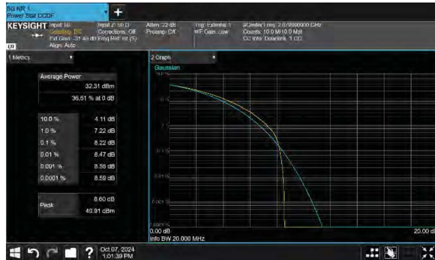
Port 1 20 MHz Channel Bandwidth QPSK Modulation High Ch, 2679.99 MHz
