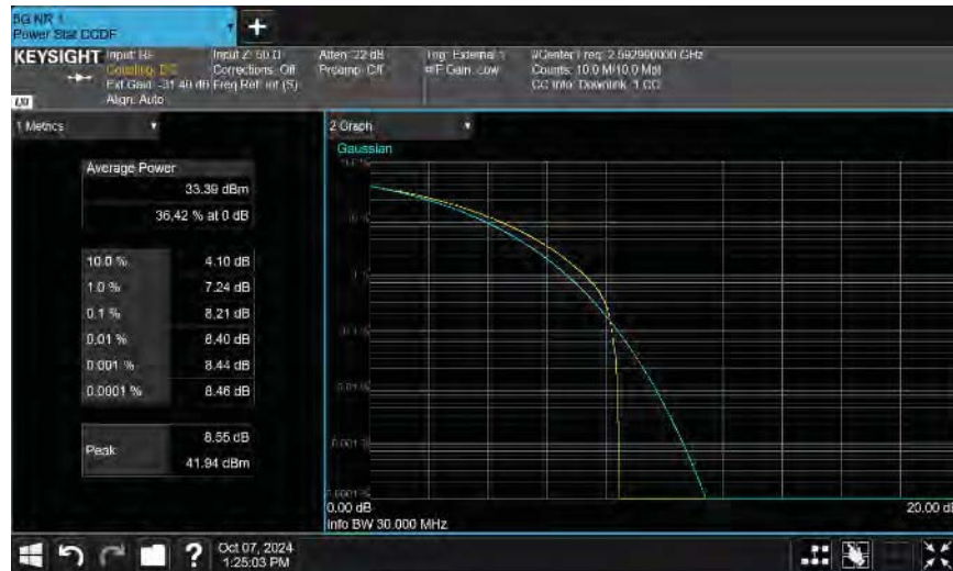
Port 1 30 MHz Channel Bandwidth QPSK Modulation Mid Channel, 2592.99 MHz
