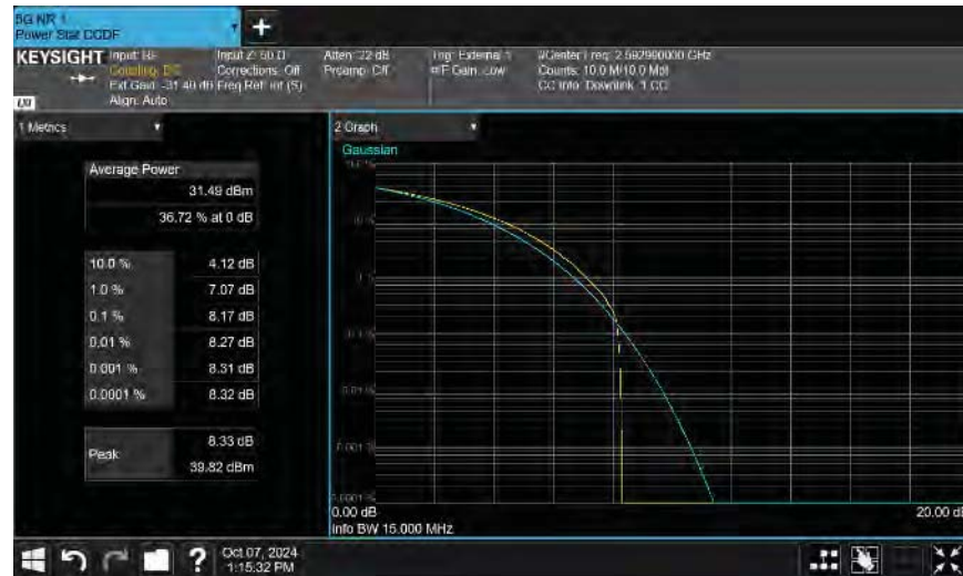
Port 1 15 MHz Channel Bandwidth QPSK Modulation Mid Channel, 2592.99 MHz
