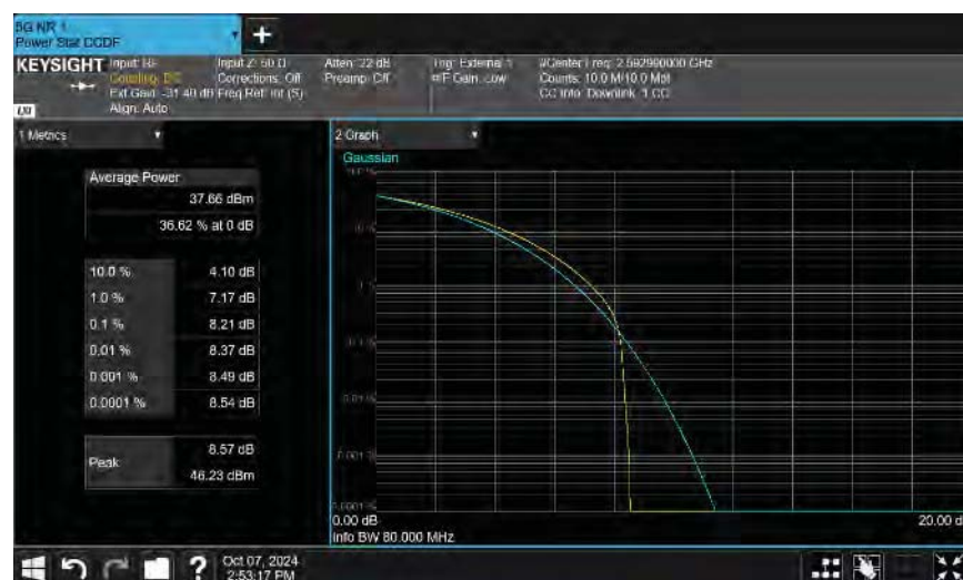
Port 1 80 MHz Channel Bandwidth 16QAM Modulation Mid Channel, 2592.99 MHz
