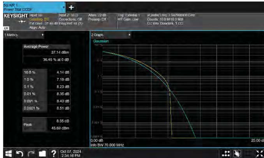
Port 1 70 MHz Channel Bandwidth QPSK Modulation Mid Channel, 2592.99 MHz
