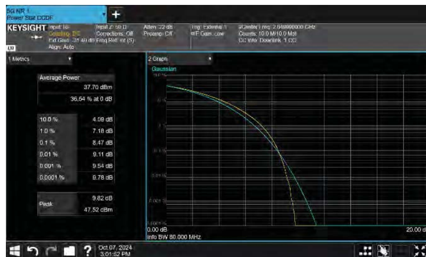
Port 1 80 MHz Channel Bandwidth QPSK Modulation High Ch, 2649.99 MHz
