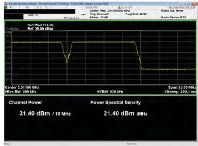
Port 1 QPSK Modulation Multicarrier Test Case 1 NR10, Low Channel, 2511.00 MHz
