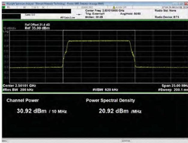
Port 1 QPSK Modulation Multicarrier Test Case 3 NR10, Low Channel, 2501.01 MHz
