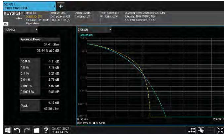
Port 1 40 MHz Channel Bandwidth QPSK Modulation Low Ch, 2516.01 MHz
