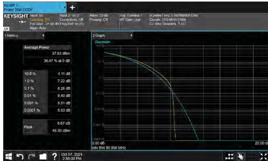
Port 1 80 MHz Channel Bandwidth 64QAM Modulation Mid Channel, 2592.99 MHz
