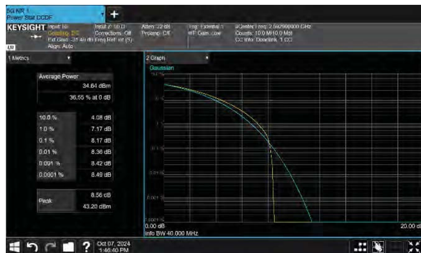
Port 1 40 MHz Channel Bandwidth QPSK Modulation Mid Channel, 2592.99 MHz
