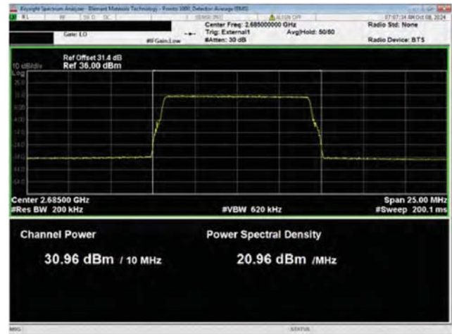
Port 1 QPSK Modulation Multicarrier Test Case 3 NR10, High Channel, 2685.00 MHz
