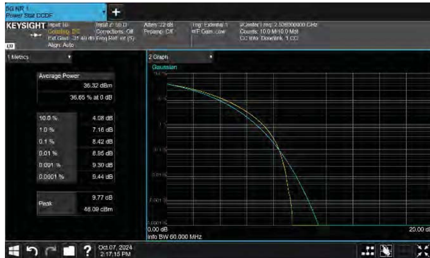
Port 1 60 MHz Channel Bandwidth QPSK Modulation Low Ch, 2526.00 MHz
