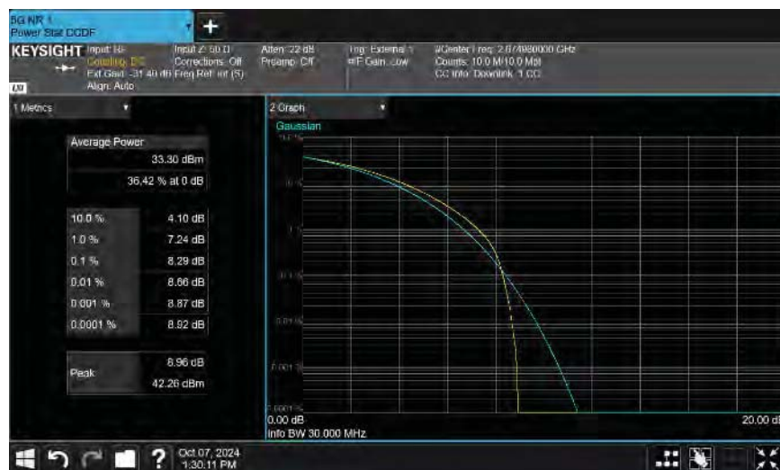
Port 1 30 MHz Channel Bandwidth QPSK Modulation High Ch, 2674.98 MHz
