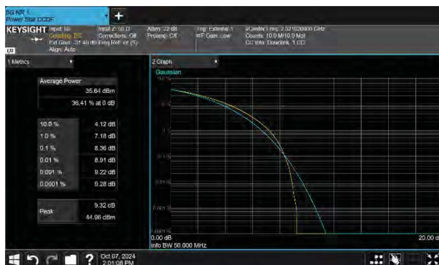
Port 1 50 MHz Channel Bandwidth QPSK Modulation Low Ch, 2521.02 MHz
