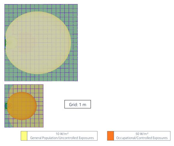
Figure 3 – Top view of the power density for the time-averaged actual maximum transmitted power of 85 W (EU/ICNIRP, Australia/NZ and US/related)
