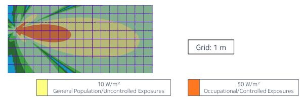
Figure 5 – Side view of the power density for the time-averaged actual maximum transmitted power of 85 W (EU/ICNIRP, Australia/NZ and US/related)
