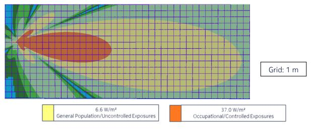
Figure 8 – Side view of the power density for the time-averaged maximum transmitted power of 339 W (Canada)
