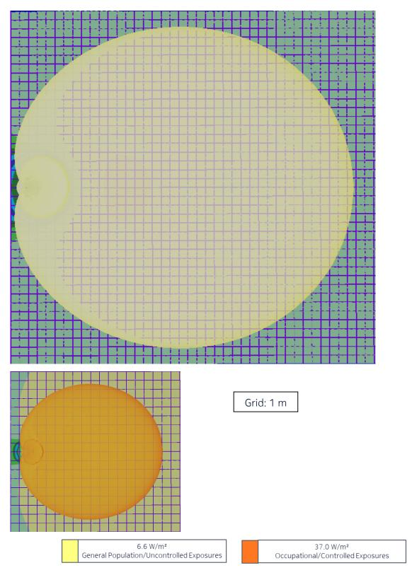
Figure 6 – Top view of the power density for the time-averaged maximum transmitted power of 339 W (Canada)
