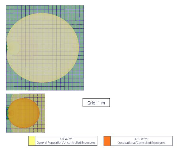
Figure 7 – Top view of the power density for the time-averaged actual maximum transmitted power of 85 W (Canada)
