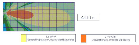
Figure 9 – Side view of the power density for the time-averaged actual maximum transmitted power of 85 W (Canada)
