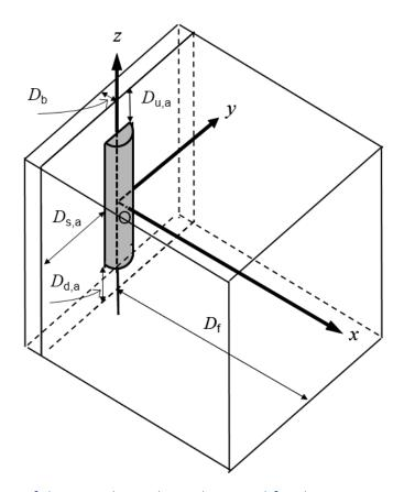
Figure 1 – Shape of the compliance boundary used for the RF exposure compliance assessment (from [4]).
