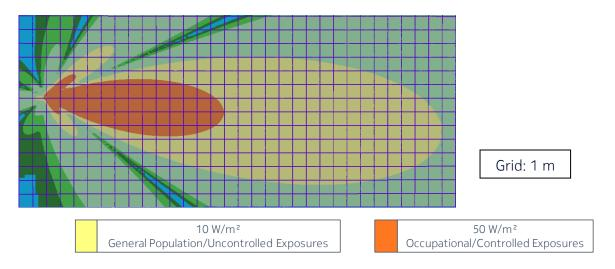
Figure 4 – Side view of the power density for the time-averaged maximum transmitted power of 339 W (EU/ICNIRP, Australia/NZ and US/related
