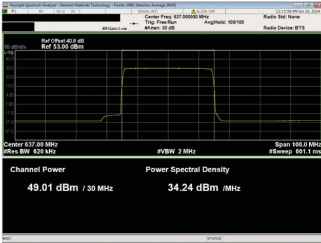
Port 1 NR 30 MHz Channel Bandwidth 64QAM High Ch, 637.0 MHz
