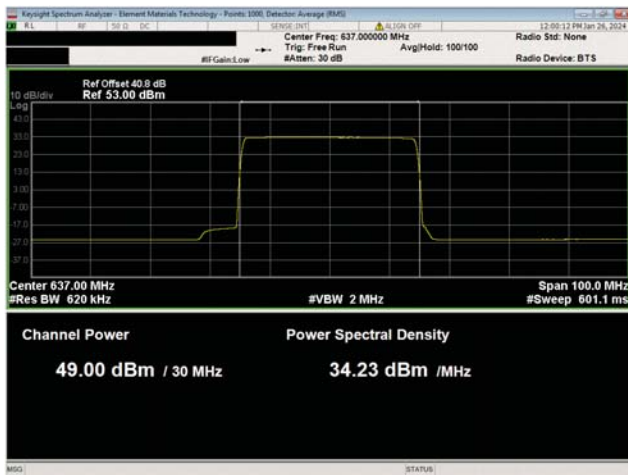
Port 1 NR 30 MHz Channel Bandwidth QPSK High Ch, 637.0 MHz
