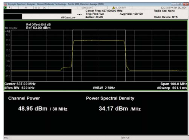
Port 1 NR 30 MHz Channel Bandwidth 256QAM High Ch, 637.0 MHz
