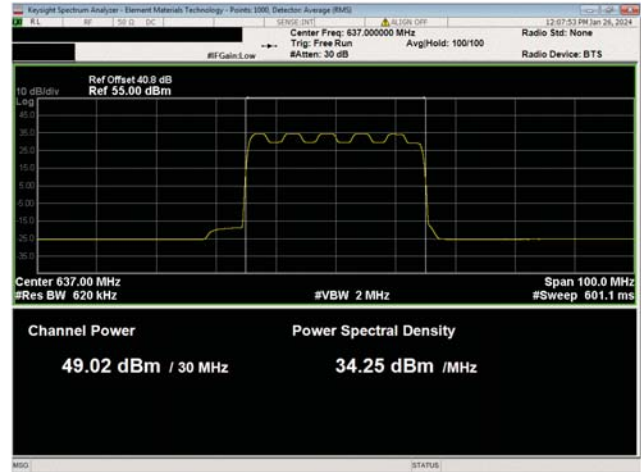
Port 1 NR 30 MHz Channel Bandwidth 16QAM High Ch, 637.0 MHz
