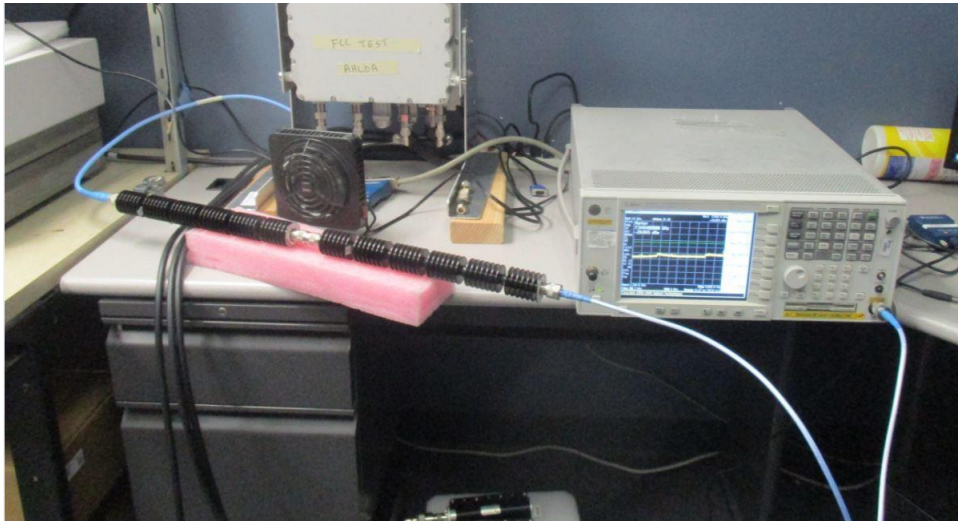
Photo of 9kHz to 150kHz, 150kHz to 20MHz, 20MHz to 600MHz, 600 to 800MHz and 800MHz to 1.2GHz Setup
