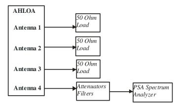
Test Setup Used for Conducted RF Measurements on AHLOA
