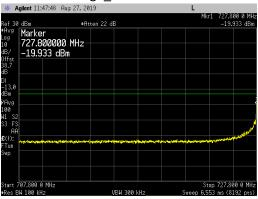
Carrier at Top Channel (745.8MHz) Upper Band Edge\_745 to 747MHz
