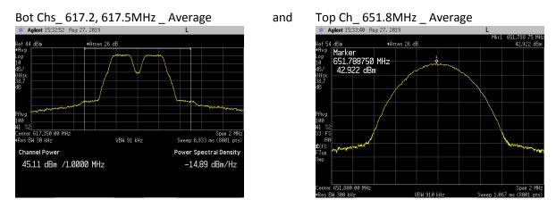
Band 71/Band 85 Three Standalone KDB 971168 Multicarrier Power Plots at Antenna Port 4:
