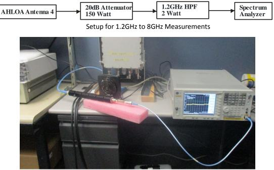
Photograph of 1.2GHz to 8GHz Test Setup
