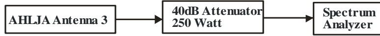
Setup for 9kHz to 150kHz, 150kHz to 20MHz and 20MHz to 1100MHz Measurements
