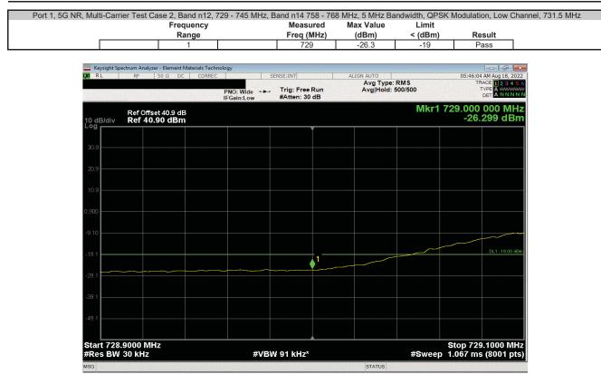
Port 1, 5G NR, Multi-Carrier Test Case 2, Band n12, 729 - 745 MHz, Band n14 758 - 768 MHz, 5 MHz Bandwidth, QPSK Modulation, Low Channel, 731.5 MHz
