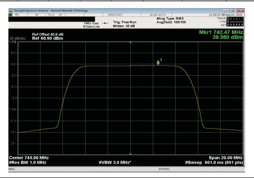
Port 1, 5G NR, Band n12, 729 - 745 Mhz, 15 MHz Bandwidth, 256QAM Modulation, Low Channel, 736.5 MHz
