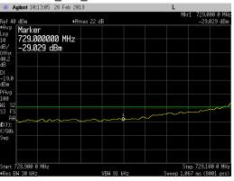
IoT Guard Band Carrier at Upper Placement Ant Port 1\_LBE\_709 to 739MHz
