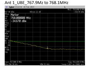
IoT Guard Band Carrier at Upper Placement
