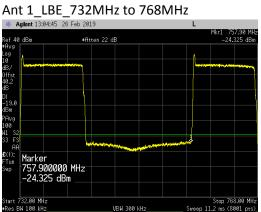
IoT Guard Band Carrier at Lower Placement
