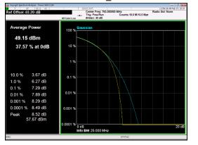
Single Narrow Band IoT Upper Guard Band Carrier: Port 1 – Middle Channel\_ CCDF
