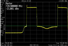
IoT Guard Band Carrier at Upper Placement Ant Port 1\_LBE\_709 to 768MHz
