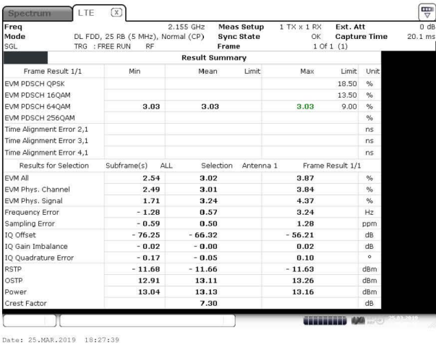
Figure 7 I/Q constellation table with I/Q error – 64QAM (2155 MHz) (5 MHz Channel BW)
