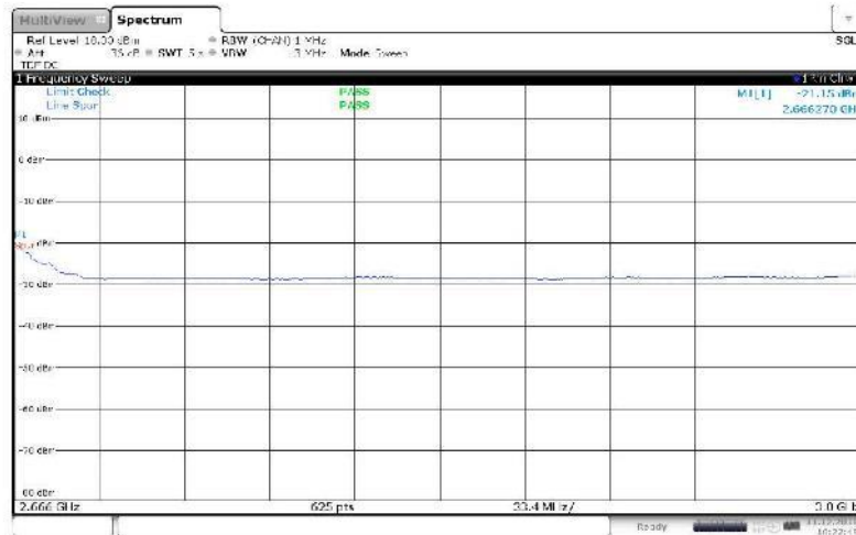
Figure 143 Spurious Emissions (9kHz – 2.644GHz) – 256QAM (2650 MHz, 2660 MHz, 2x10 MHz Channel BW)
