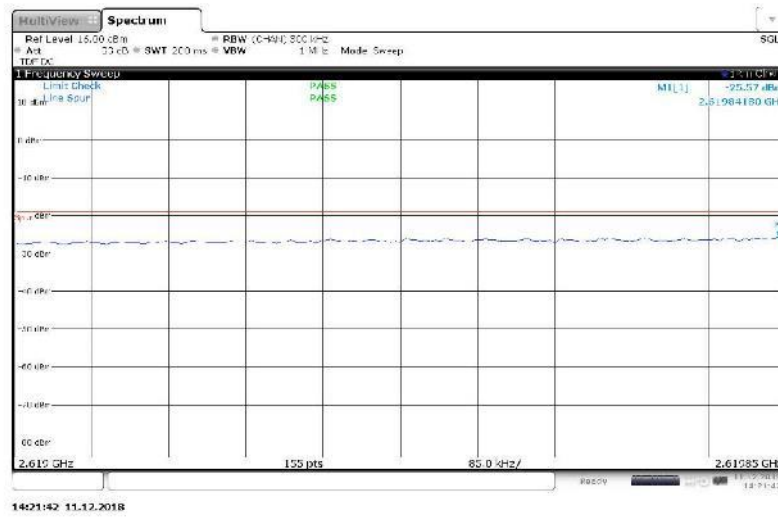
Figure 147 Spurious Emissions (Lower Band Edge) – QPSK (2627.5 MHz, 2642.5 MHz, 2x15 MHz Channel BW)
