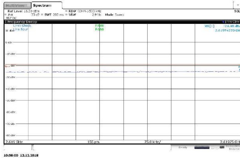
Figure 183 Spurious Emissions (Lower Band Edge) – 64QAM (2630 MHz, 2650 MHz, 2x20 MHz Channel BW)
