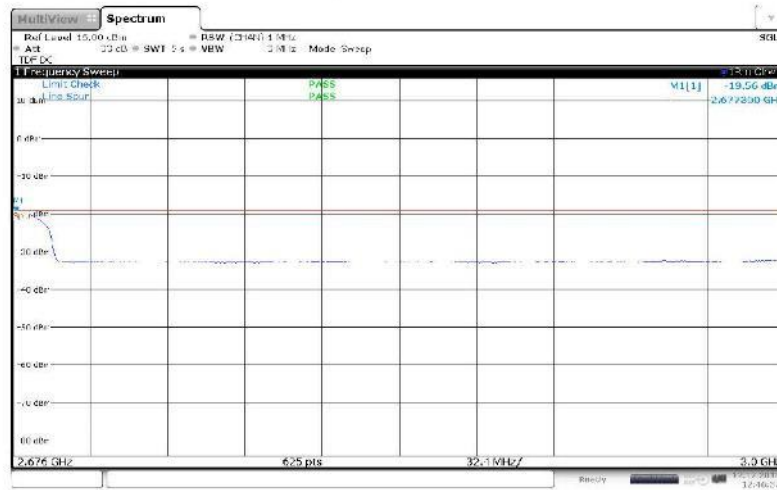
Figure 174 Spurious Emissions (2.676 GHz – 3 GHz) – QPSK (2645 MHz, 2665 MHz, 2x20 MHz Channel BW)
