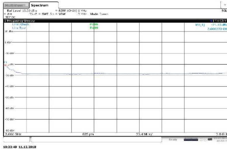
Figure 144 Spurious Emissions (2.666 GHz – 3 GHz) – 256QAM (2650 MHz, 2660 MHz, 2x10 Channel BW)
