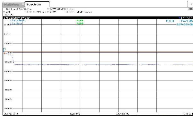
Figure 191 Spurious Emissions (9kHz – 2.634GHz) – 256QAM (2645 MHz, 2665 MHz, 2x20 MHz Channel BW)
