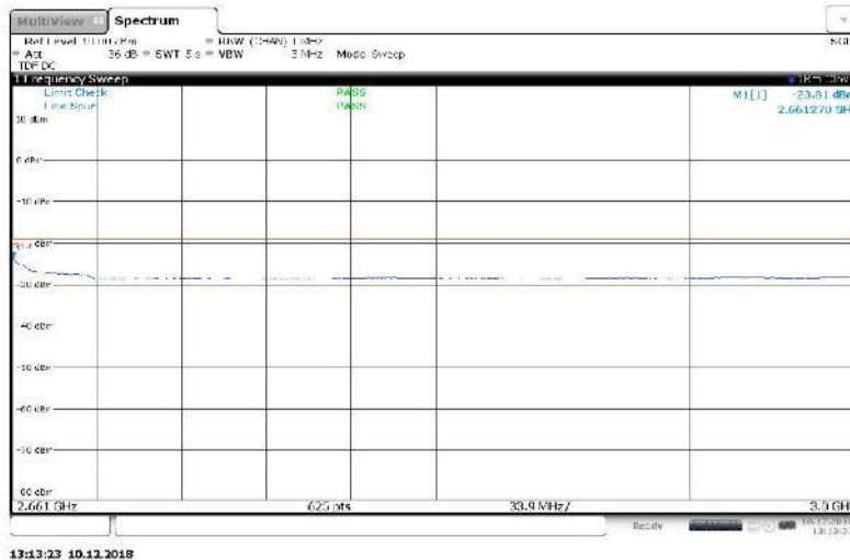
Figure 108 Spurious Emissions (2.661 GHz – 3 GHz) – 16QAM (2652.5 MHz, 2657.5 MHz, 2x5 Channel BW)
