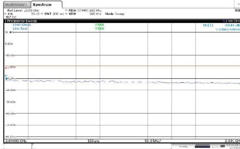
Figure 45 Spurious Emissions (Lower Band Edge) – 256QAM (2625 MHz, 10 MHz Channel BW)
