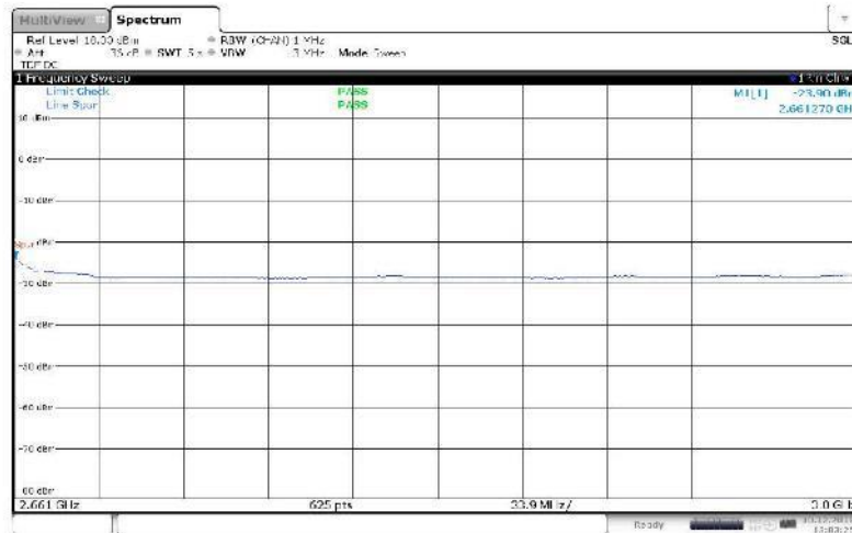
Figure 113 Spurious Emissions (9kHz – 2.649GHz) – 64QAM (2652.5 MHz, 2657.5 MHz, 2x5 MHz Channel BW)
