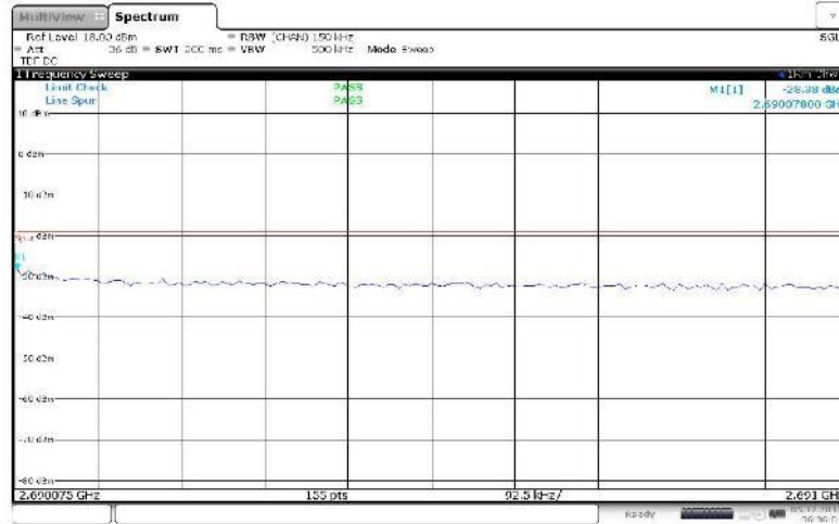
Figure 57 Spurious Emissions (Lower Band Edge) – 16QAM (2627.5 MHz, 15 MHz Channel BW)
