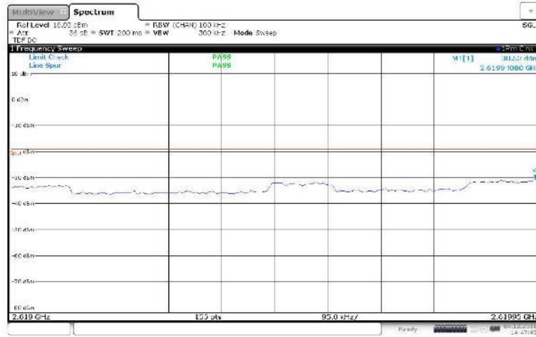
Figure 45 Spurious Emissions (Lower Band Edge) – 256QAM (2625 MHz, 10 MHz Channel BW)
