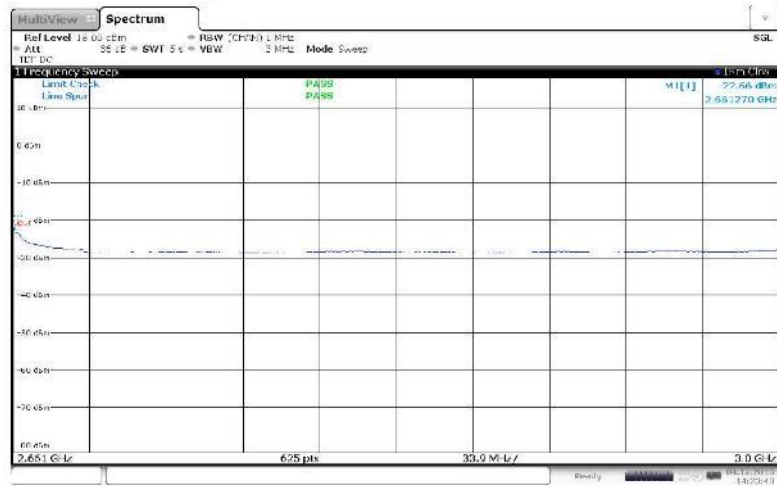
Figure 29 Spurious Emissions (9kHz – 2.649 GHz) – QPSK (2655 MHz, 10 MHz Channel BW)
